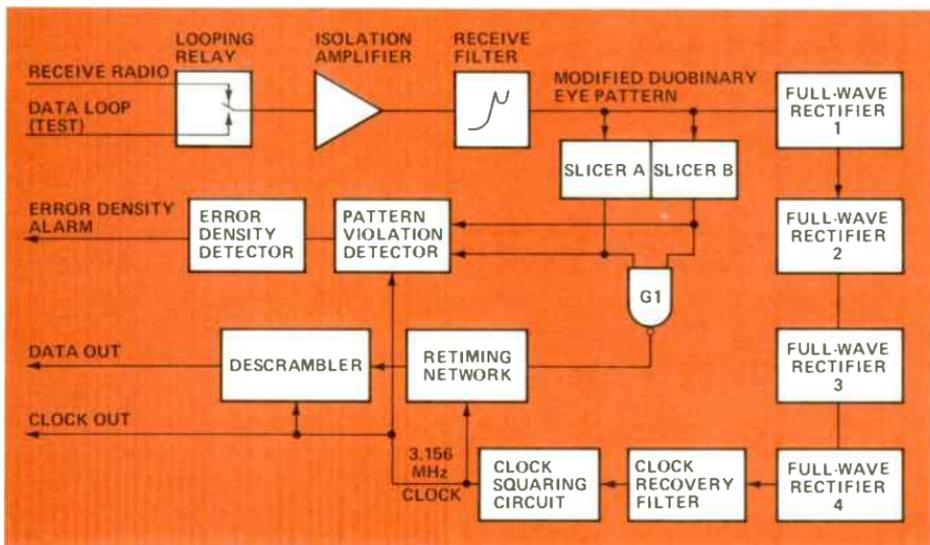
Figure 5. The receive interface unit completes the conversion to modified duobinary, recovers the clock, and descrambles the incoming signal.
