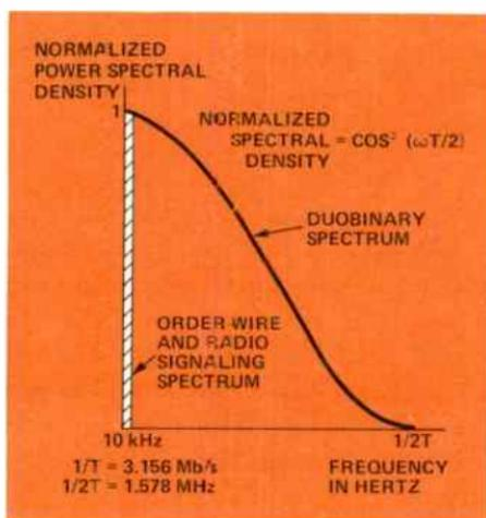
Figure 1. The conflicting spectrums of order wire and duobinary require modification of the duobinary waveform.
