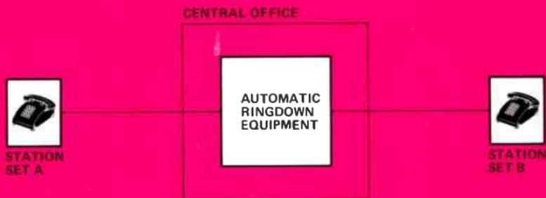
*Figure 4. An automatic ringdown private line allows one station to ring the other as soon as the handset is lifted. One application of this service is in airports and similar facilities to summon taxicabs and make hotel reservations.*
