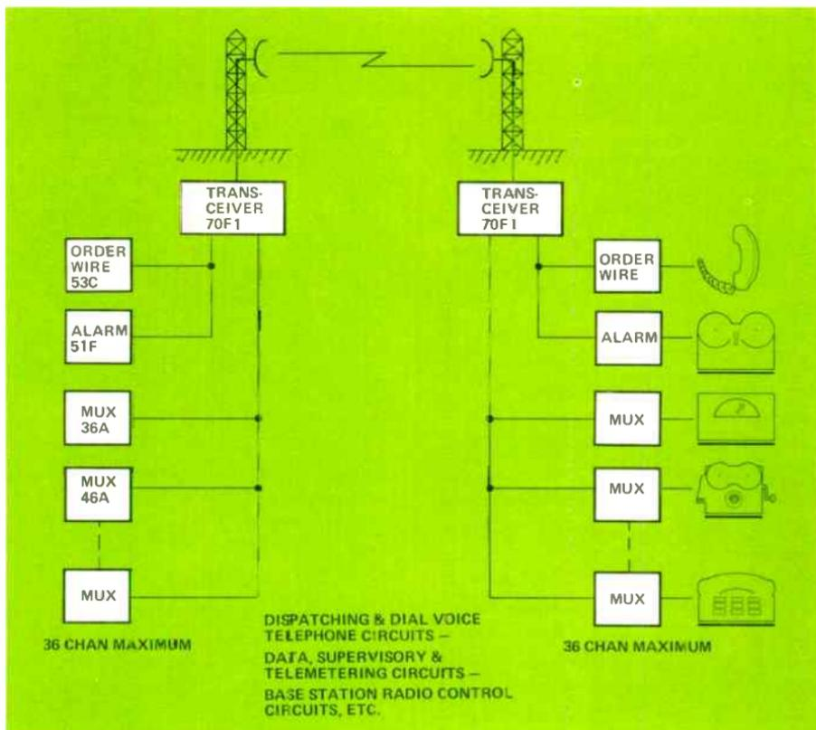
Figure 2. Typical layout of a light-route radio system.
