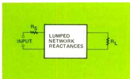
Figure 10. A filter network is essentially a group of reactances terminated by a load ( $R_L$ ) and source ( $R_S$ ) resistance. Unlike an image parameter-designed filter, the terminations in synthesis design are not constrained to match the network impedance characteristic.
