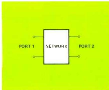
Figure 3. A four-terminal network has two ports, either of which may be used as an input point.
