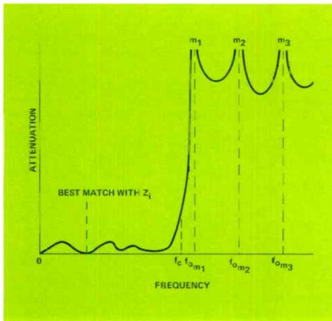
Figure 8. The pass-band response of an image parameter-designed filter may exhibit an arbitrary ripple shape, as shown in this response curve for an  $m$ -derived filter with three  $m$ -resonant components.
