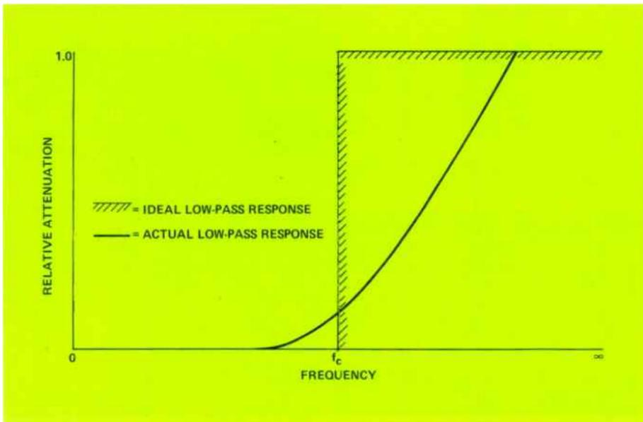
Figure 2. Low-pass filters reject signals above a specific cut-off frequency ( $f_c$ ) by providing increased attenuation. The ideal is instant rejection at  $f_c$ ; the actuality is a curve increasing with frequency.
