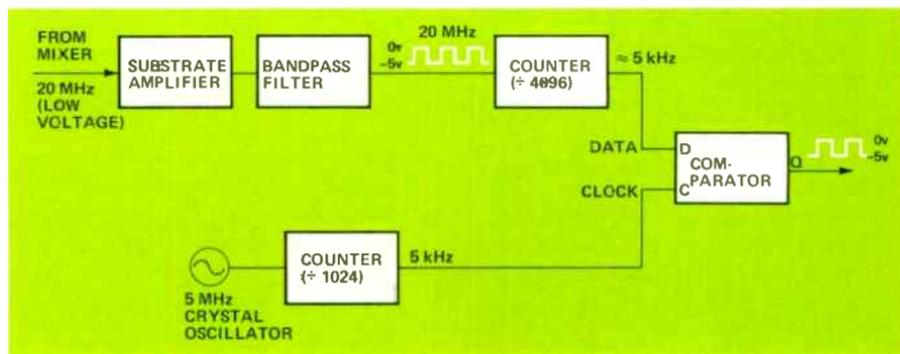
Figure 5. The basic components of the digital afc.
