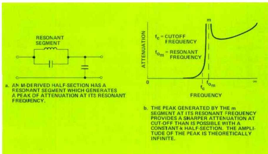
Figure 6. The  $m$ -derived filter is the most common image parameter design because of its attenuation peaks. By joining half-sections into a complex filter, several peaks can be established to make optimum use of the stopband with minimum physical components.
