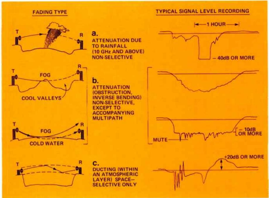
Figure 3. Non-selective fading types.
