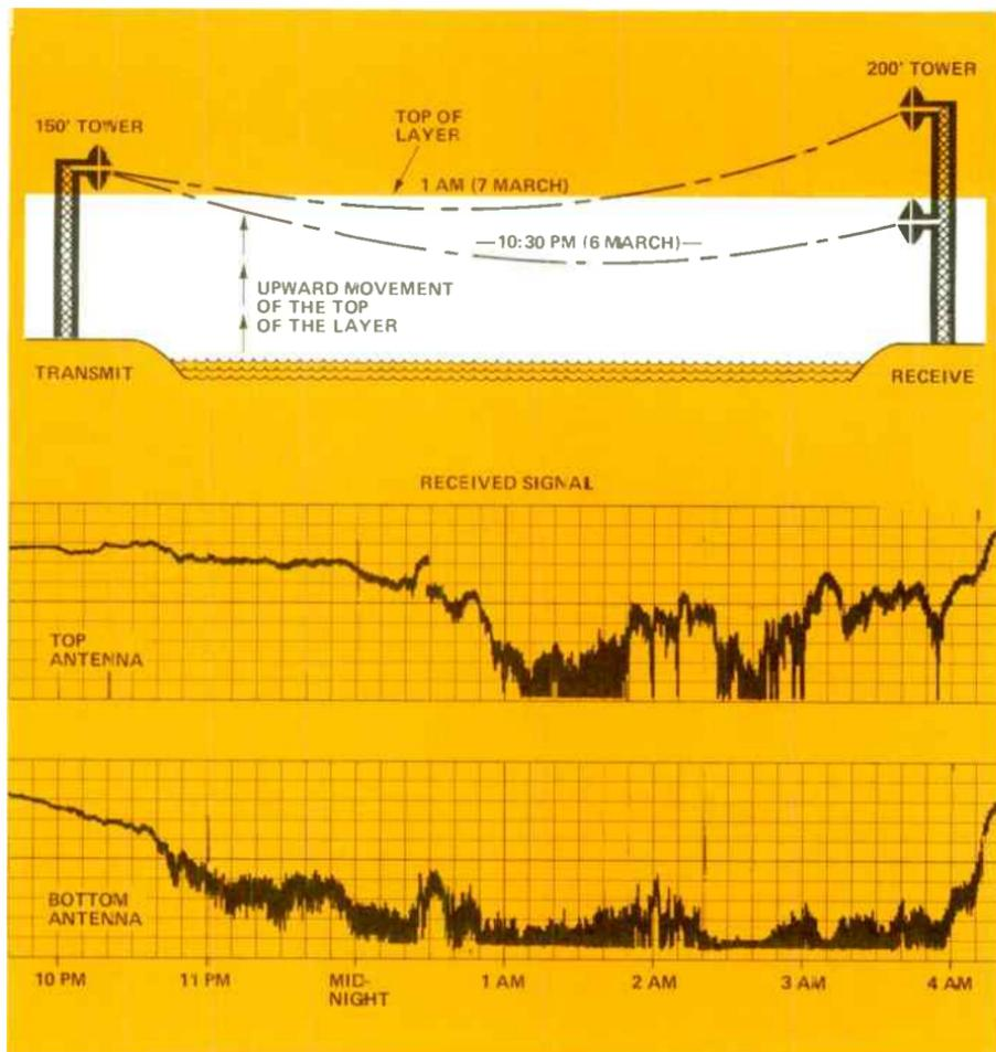
Figure 3. Blackout fading on both space diversity antennas.
