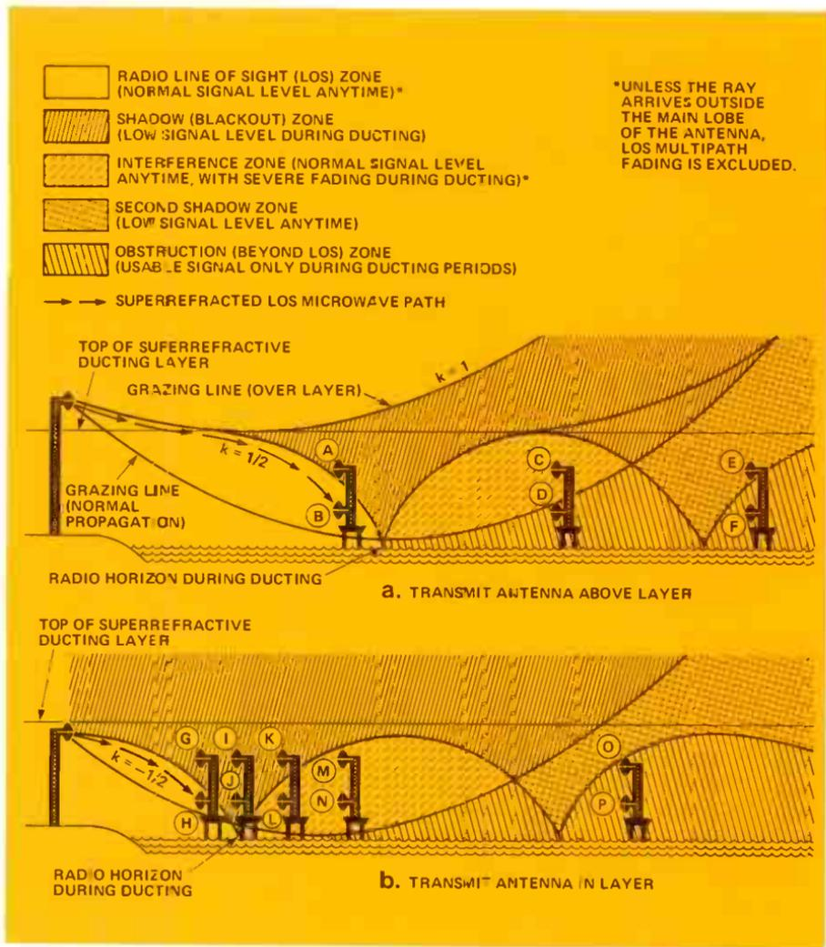
Figure 1. Tracing of a microwave beam within a superrefractive ground-based layer with (a) transmit antenna above layer and (b) transmit antenna in layer.
