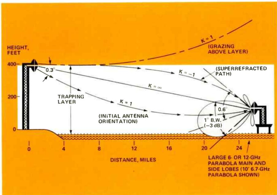
Figure 4. Antenna decoupling in a superrefractive ground-based layer.
