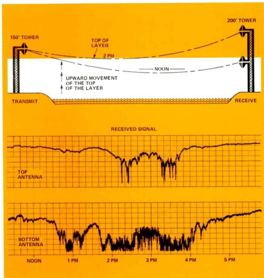
Figure 2. Blackout fading on lower space diversity antenna.
