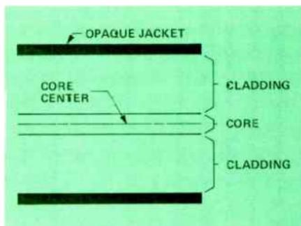
Figure 7. The step-index single-mode optical fiber must be used with the coherent light from a laser.
