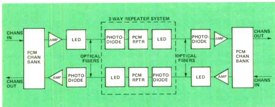
Figure 8. A simple, hypothetical optical communications system using currently available PCM equipment.
