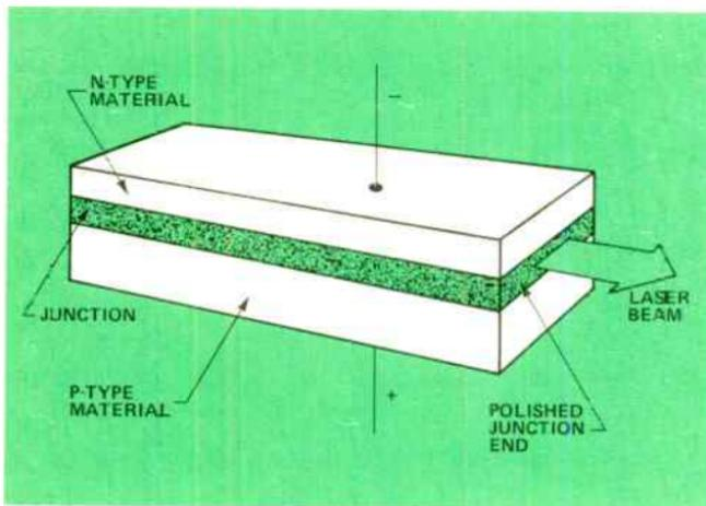
Figure 5. Principal elements of the injection laser.
