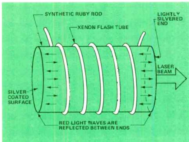
*Figure 4. Theodore Maiman's first laser had silver coatings on the ends of the ruby rod; later adaptations of the device utilized external silver mirrors at the ends of the rods.*
