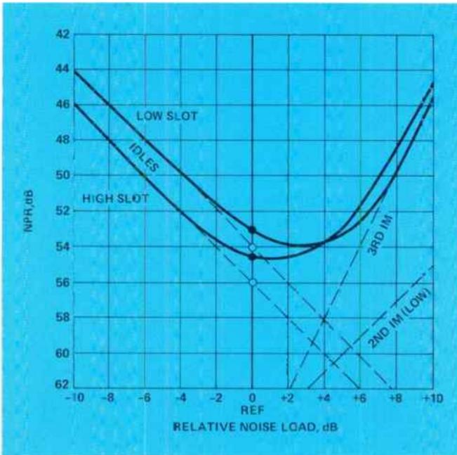
Figure 18. Excessive low-slot idle noise caused by a noisy amplifier or waveguide conversion product.
