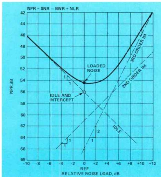
Figure 6. The NPR (bucket) curve, with radio-only noise or distortion elements.
