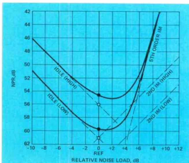
Figure 11. Same as Figure 10, but with 5th order IM establishing the higher order tangent line.
