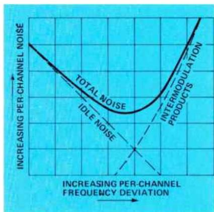
Figure 4. An optimum balance between idle and IM noise contributions is desired in a microwave system.
