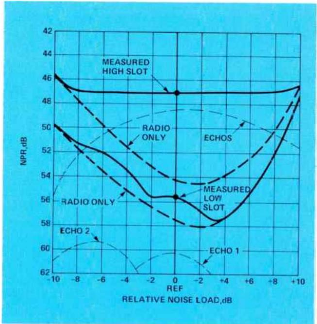
Figure 10. Typical high-slot noise load curve for a 6-hop baseband microwave system.
