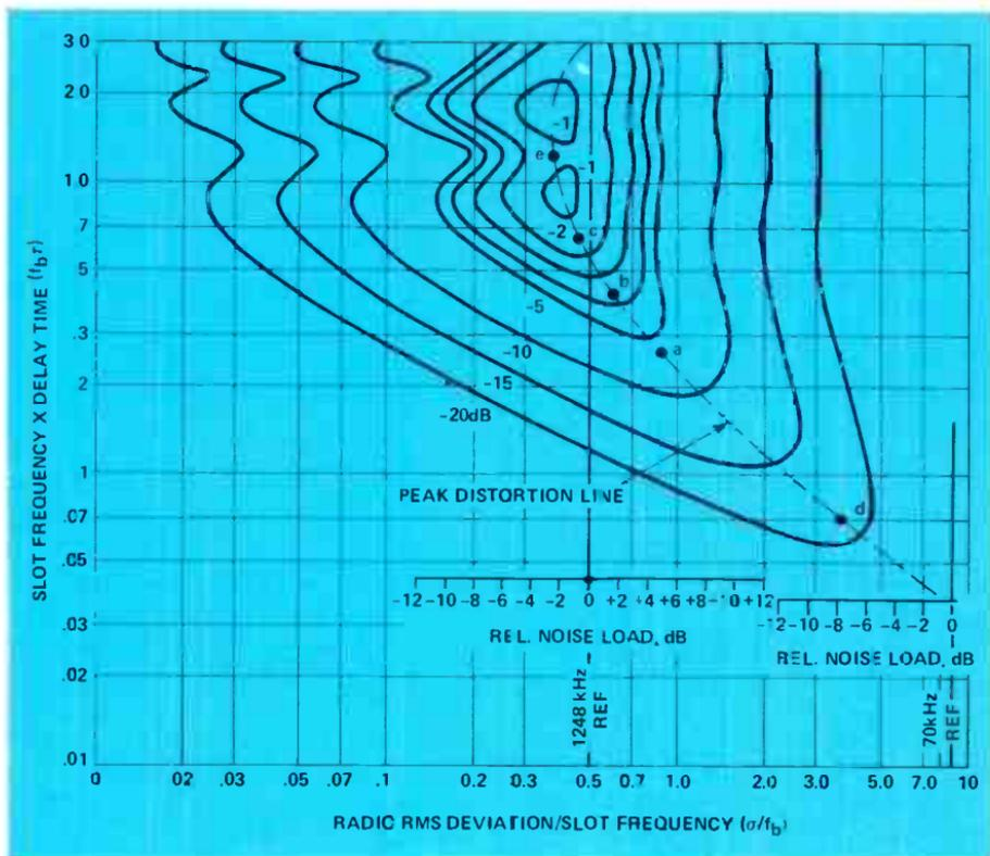
Figure 7. Contours of constant echo amplitude-to-echo distortion ratio.
