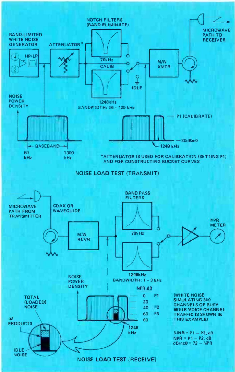
Figure 2. A typical white noise load measurement test setup.
