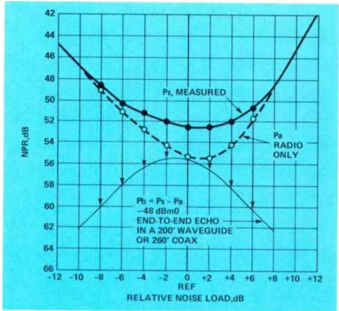
The inverse parabola, plotted by subtracting the radio-only noise (the sum of the idle, 2nd order, and higher order lines) from the measured bucket curve, does not differentiate between the four echo distortion contributors listed above, except in that far-field path IM will cause loaded noise readings to fluctuate rapidly over a wide range (1-10 dB or more).
