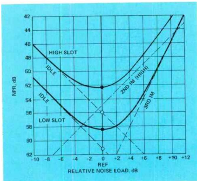
Figure 2. Excessive high-slot 2nd order IM distortion requiring delay slope equalization.
