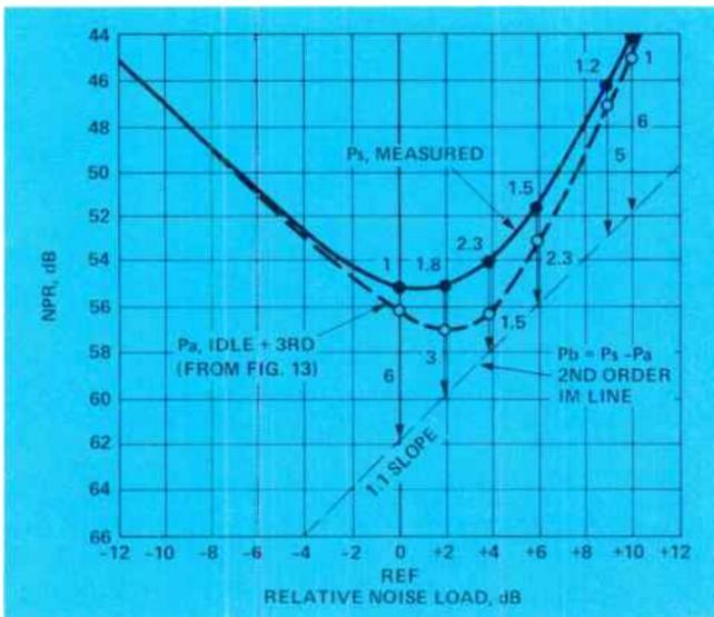
Figure 14. The second step in computing the 2nd order IM line is to subtract the sum of the tangents from the measured (total) noise (no echo distortion).
