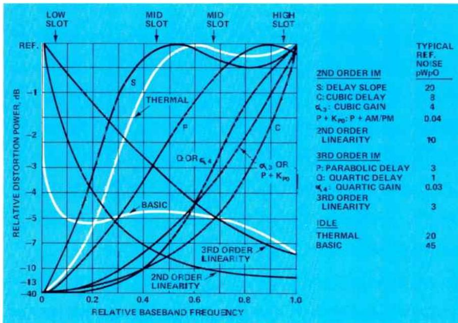
Figure 7. Distribution of distortion power in a typical baseband microwave link (with emphasis).
