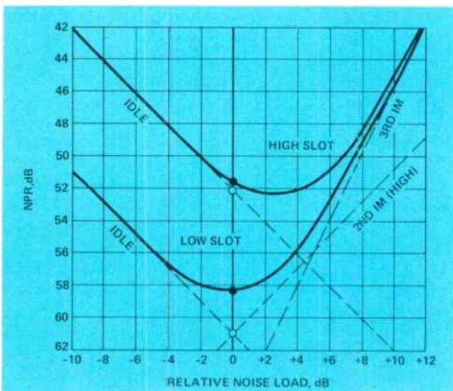
Figure 17. Excessive high-slot idle noise with a depressed rf input signal level.
