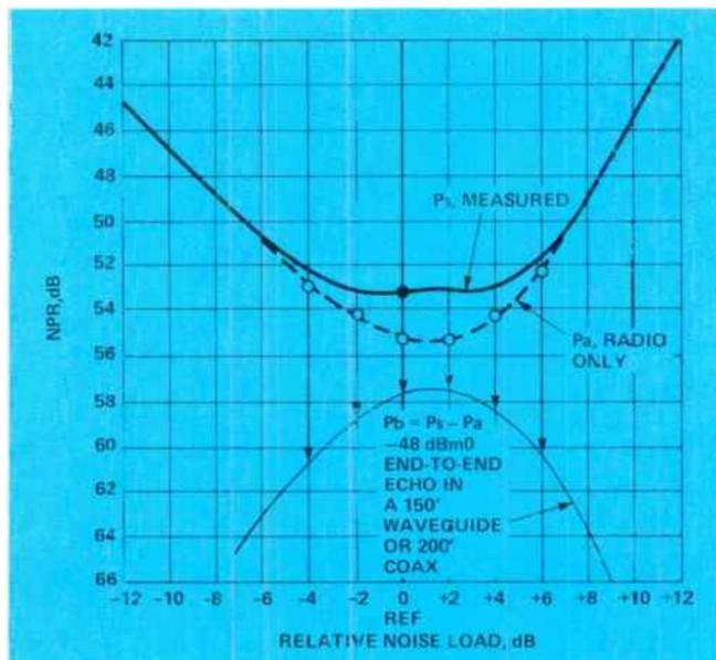
Figure 5. Same as Figure 4, but with a 150-foot waveguide echo.
