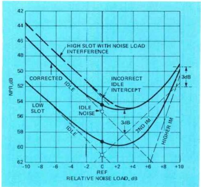
Figure 10. Bucket curves showing the idle and 3rd order tangent lines.
