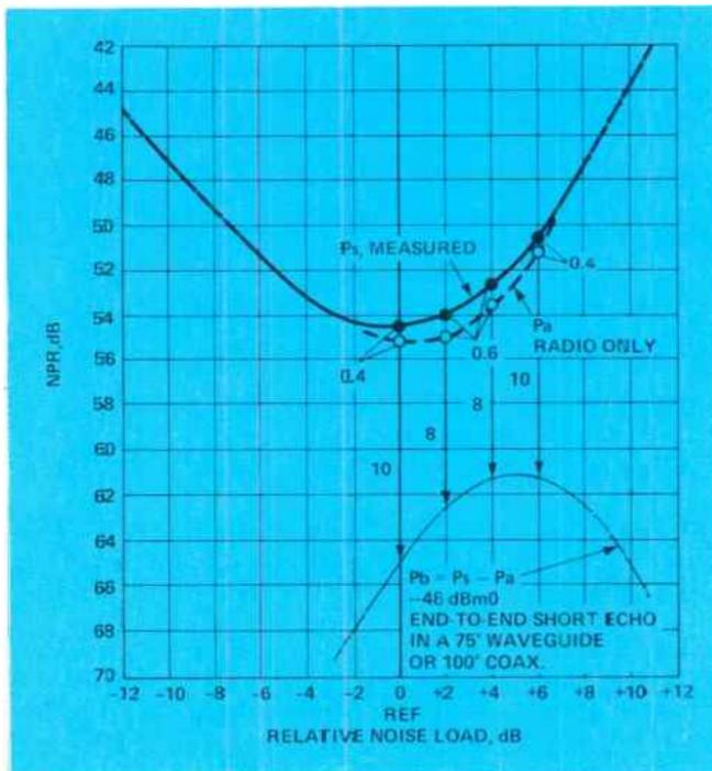
Figure 4. The radio-only bucket is subtracted from the measured total system noise curve to derive the echo distortion contribution.
