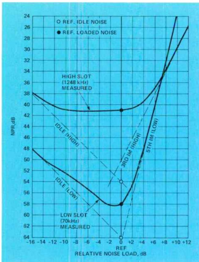
Figure 11. Bucket curves for a microwave link with excessive high-slot noise.
