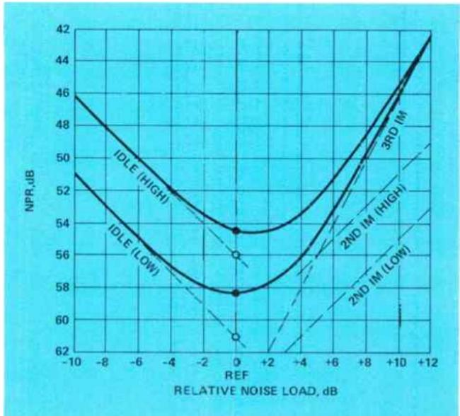
If this precaution is taken, an idle line drawn at 45° from the upper left to the lower right tangential to the bucket curve should intercept the idle noise point. The interception of this idle line with the reference noise load line is the “idle intercept point,” and
