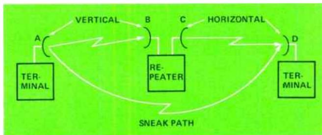
Figure 7. Cross-polarization of antennas can reduce the effects of delay distortion caused by "sneak" paths.
