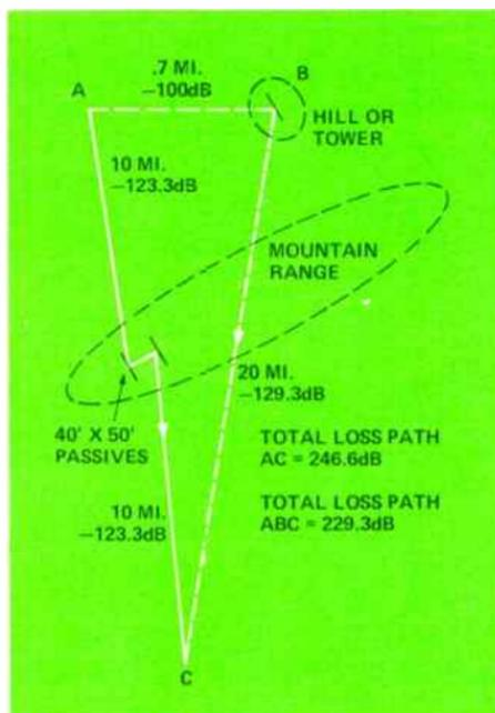
Figure 6. An rf repeater offers improved gain and economy in straight-line path narrowband applications.
