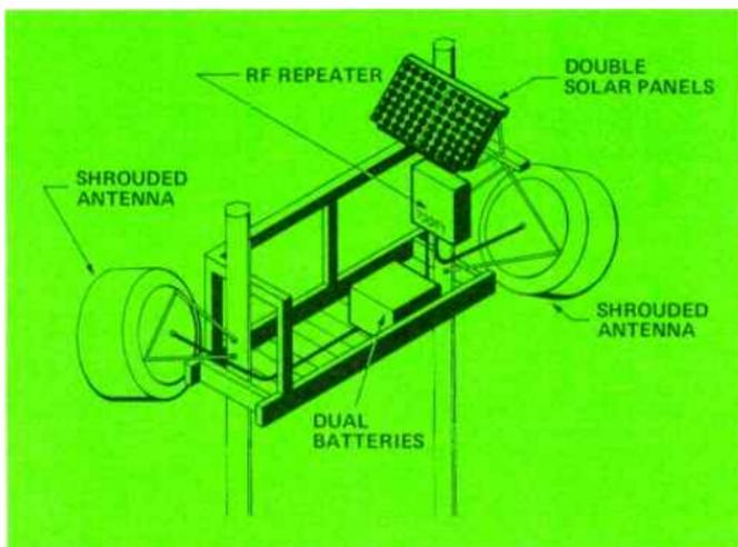
long hops as an economy measure. In flat terrain, for example, where a path between baseband repeaters may be 30 to 40 miles, 300-to-400 foot towers are usually required. By placing an rf repeater at approximately 20 miles, the tower height requirements for the baseband repeaters would then be only 100 to 200 feet, thus saving the high cost of erecting tall towers. The cost savings in this application is substantial due to the low price of the rf repeater.
