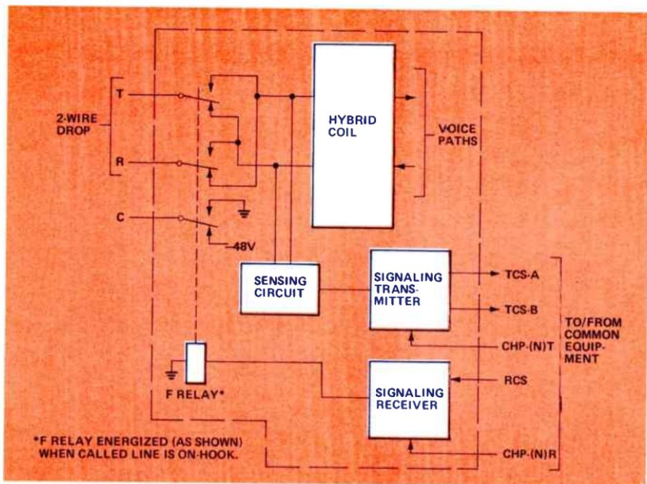
Figure 4. Basic dial pulse originating (DPO) channel unit signaling circuitry.
