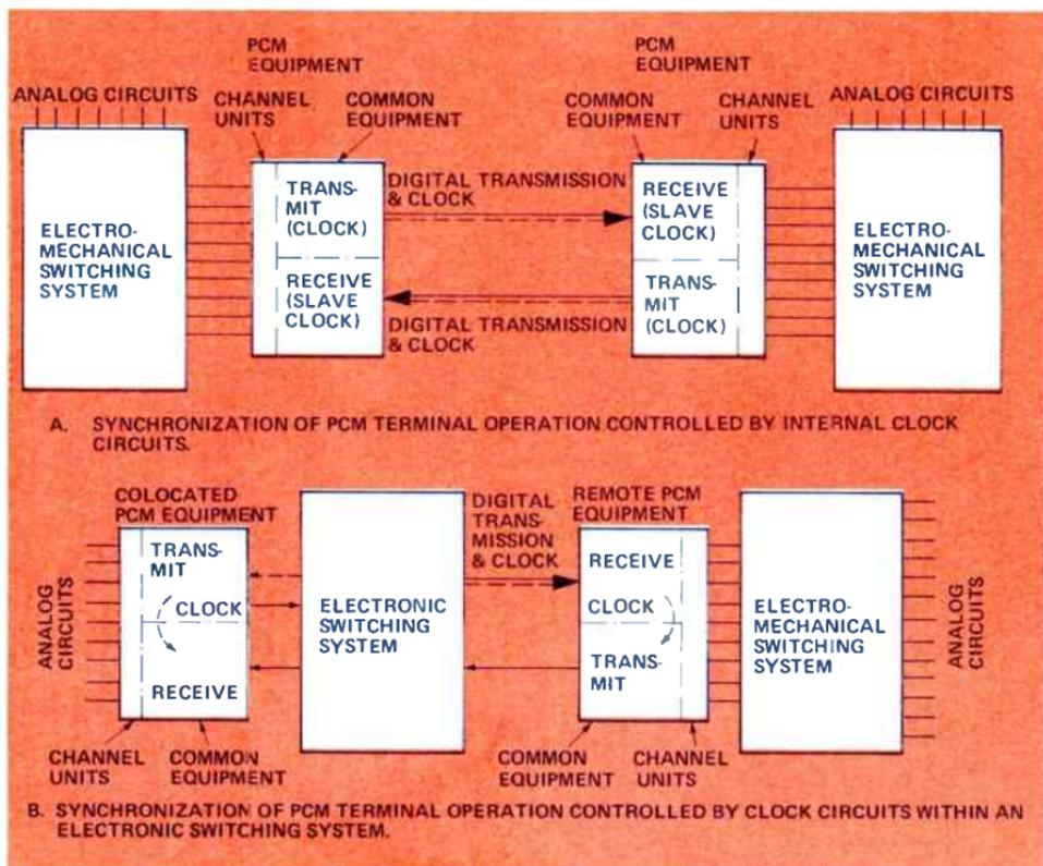
Figure 11. Timing control is essential in systems utilizing PCM techniques, and it can be implemented in several ways, depending upon the network configuration.
