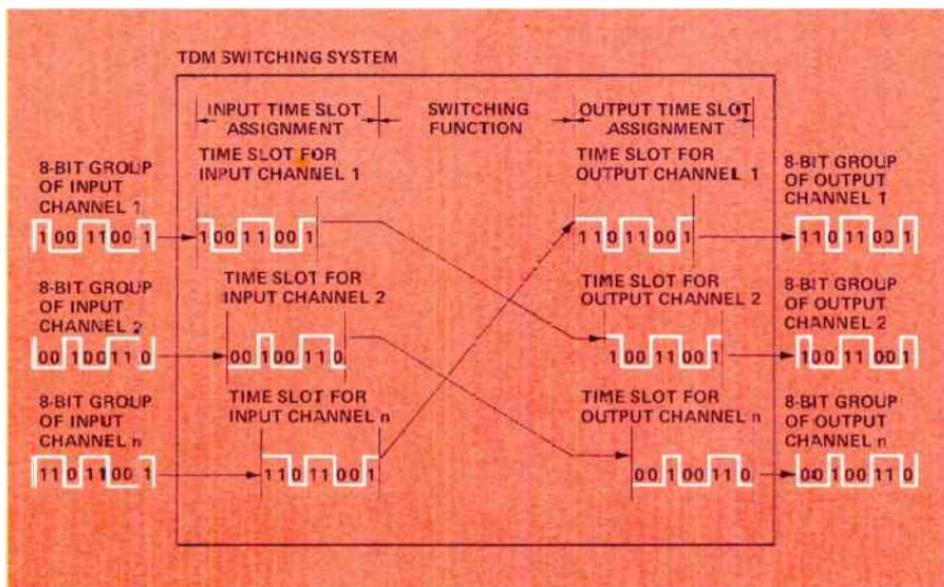
*Figure 9. In TDM switching, input and output channels are associated with unique time slots. The switching process involves transferring the contents of one slot into the desired output channel slot.*
