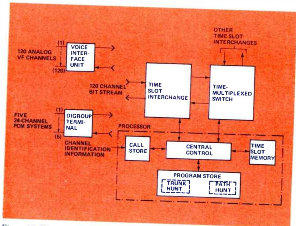
Figure 10. Electronic switching using a time-space-time configuration.
