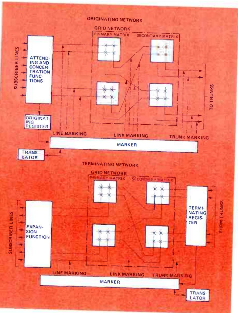
Figure 6. A simplified two-stage register-marker system in which origination and termination are accomplished in separate networks.
