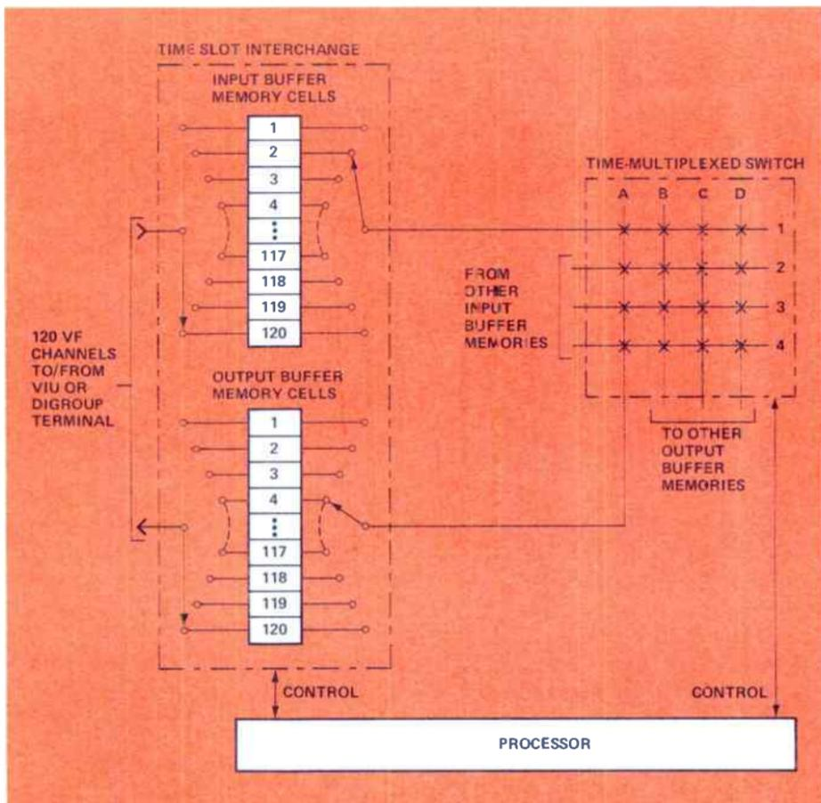
Figure 11. In a time-space-time switching configuration, input memory cells are read into output memory cells through a solid-state matrix under the direction of a computer-like processor. The process is carried out by rearranging binary words in time and space; the rotary switch symbol is used only for the sake of convenience.
