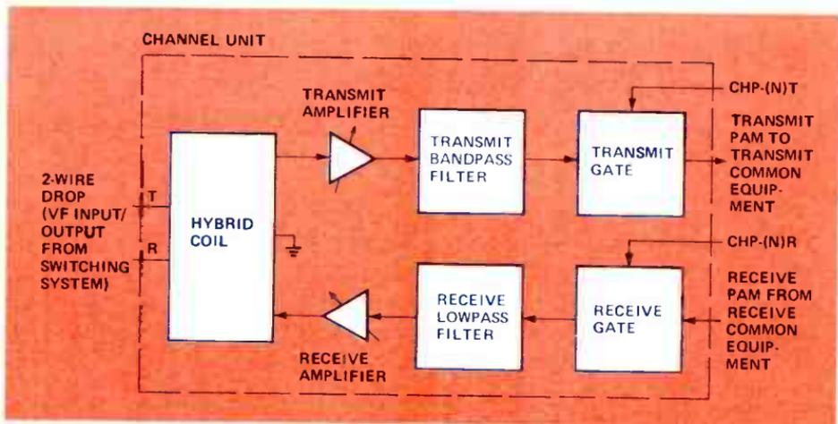
Figure 3. The transmit and receive vf paths through a channel unit typically involve a 2-wire-to-4-wire conversion and an analog/PAM interface.
