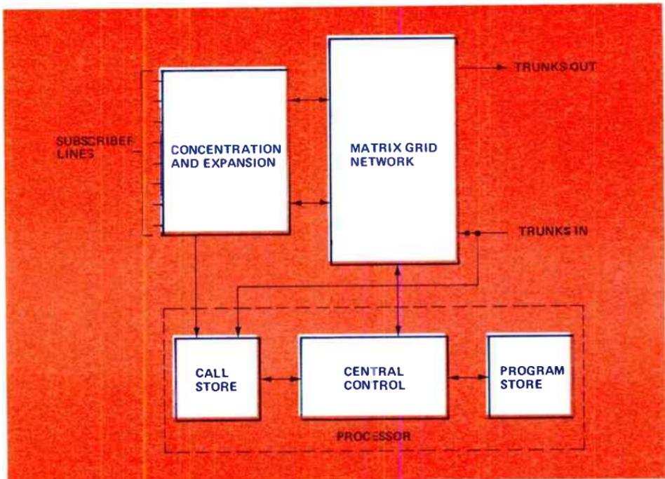
Figure 8. In electronic stored-program switching systems, control is exercised by a computer-like processor.
