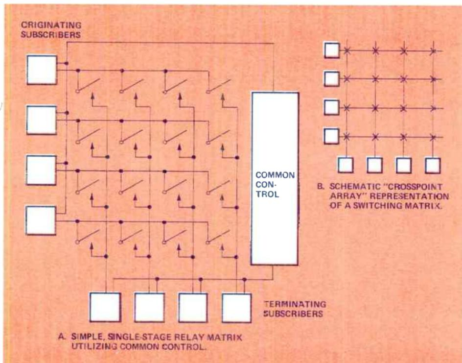
Figure 5. A switching matrix, or crosspoint array, provides connection between subscribers, and is the basic element in non-progressive networks.
