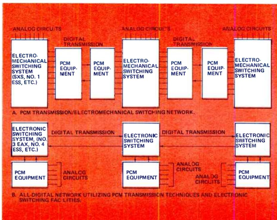
Figure 10. Analog signals must undergo a number of conversions in passing through a PCM/electromechanical network, but would need to be converted twice in an all-digital network.
