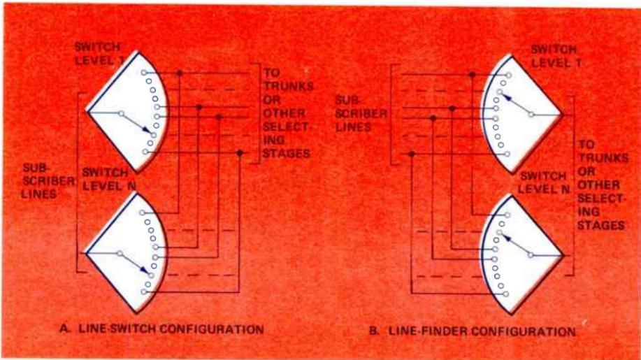
Figure 2. Concentration stages are typically of the line-switch or line-finder variety.
