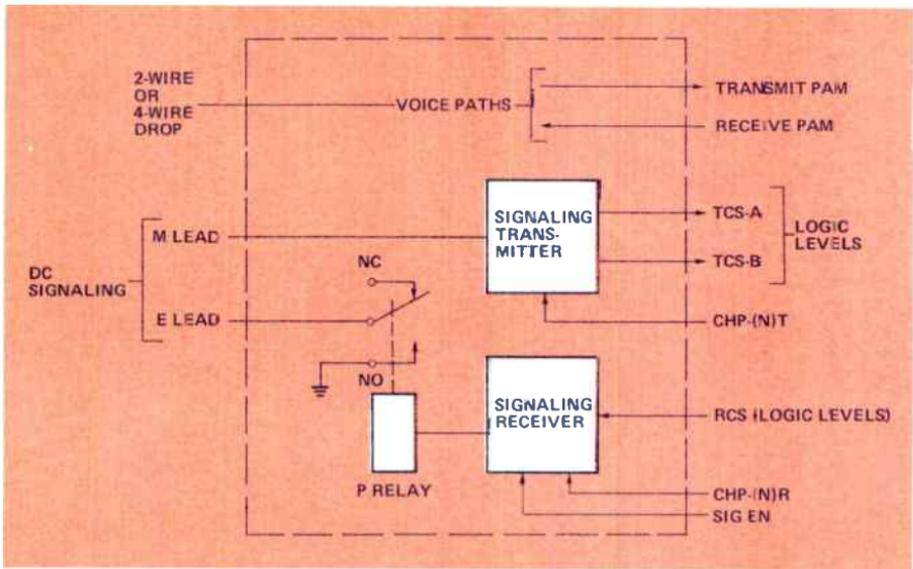
Figure 7. Basic F&M signaling channel unit circuitry.
