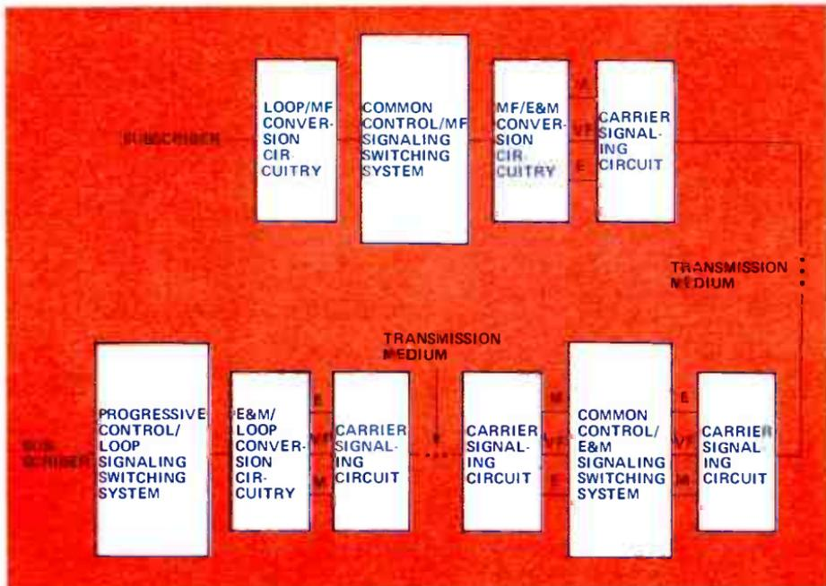
Figure 8. A telephone call may have to pass through a series of different switching systems and undergo a number of signaling format conversions.
