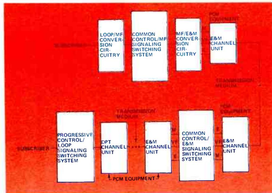
Figure 9. PCM systems can ease the problem of interfacing diverse switching systems.
