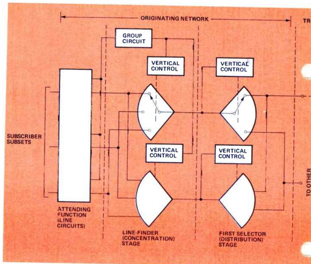
Figure 3. In a direct progressive system, electrical pulses generated by a subscriber subset directly control the switching action.
