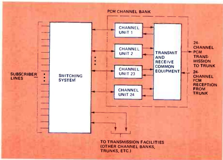
Figure 2. To increase the capacity of a transmission facility, the interface of a switching system and its trunks can include a PCM channel bank.
