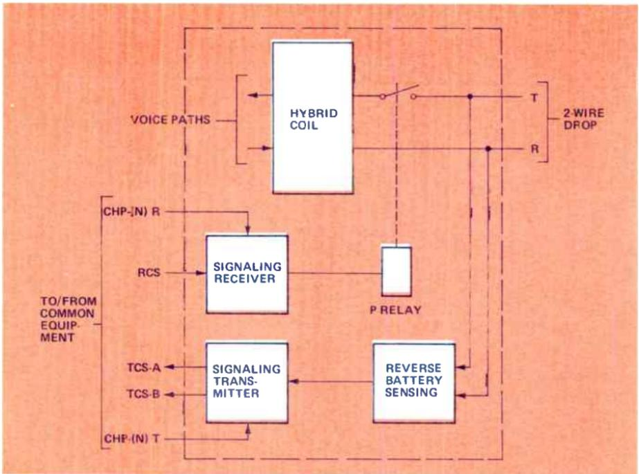
Figure 5. Basic dial pulse terminating (DPT) channel unit signaling circuitry.
