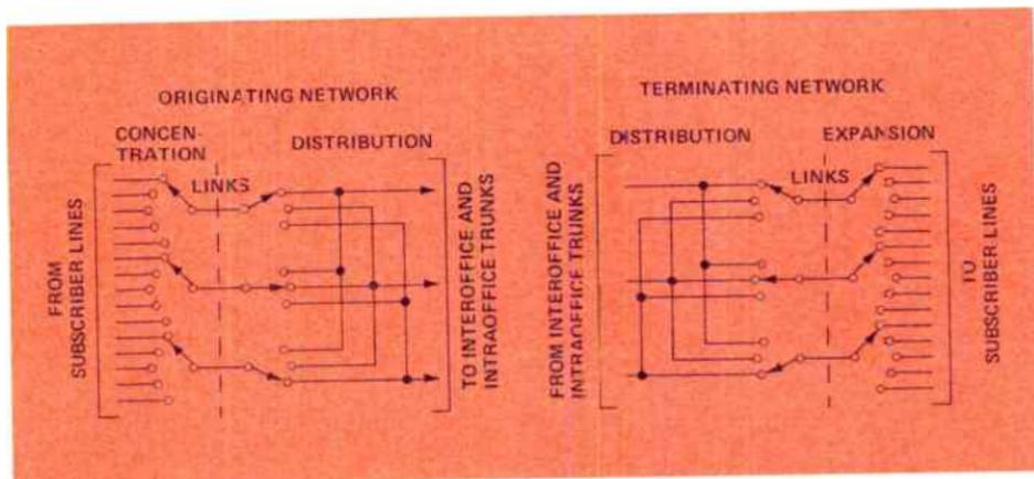
Figure 1. Concentration, distribution and expansion stages in a switching system allow a limited number of trunks to serve a larger number of subscribers.
