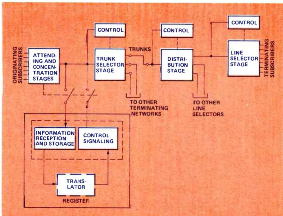
Figure 4. In a register progressive system, the subscriber is isolated from the control function by a register, in which dial pulses are translated into a form more compatible with electromechanical switch operation.
