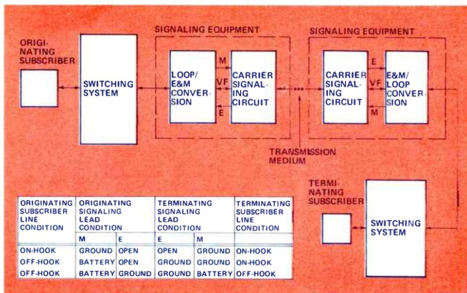
Figure 6. In a typical E&M circuit application, battery, ground and open conditions are conveyed simultaneously in both directions on E and M leads.
