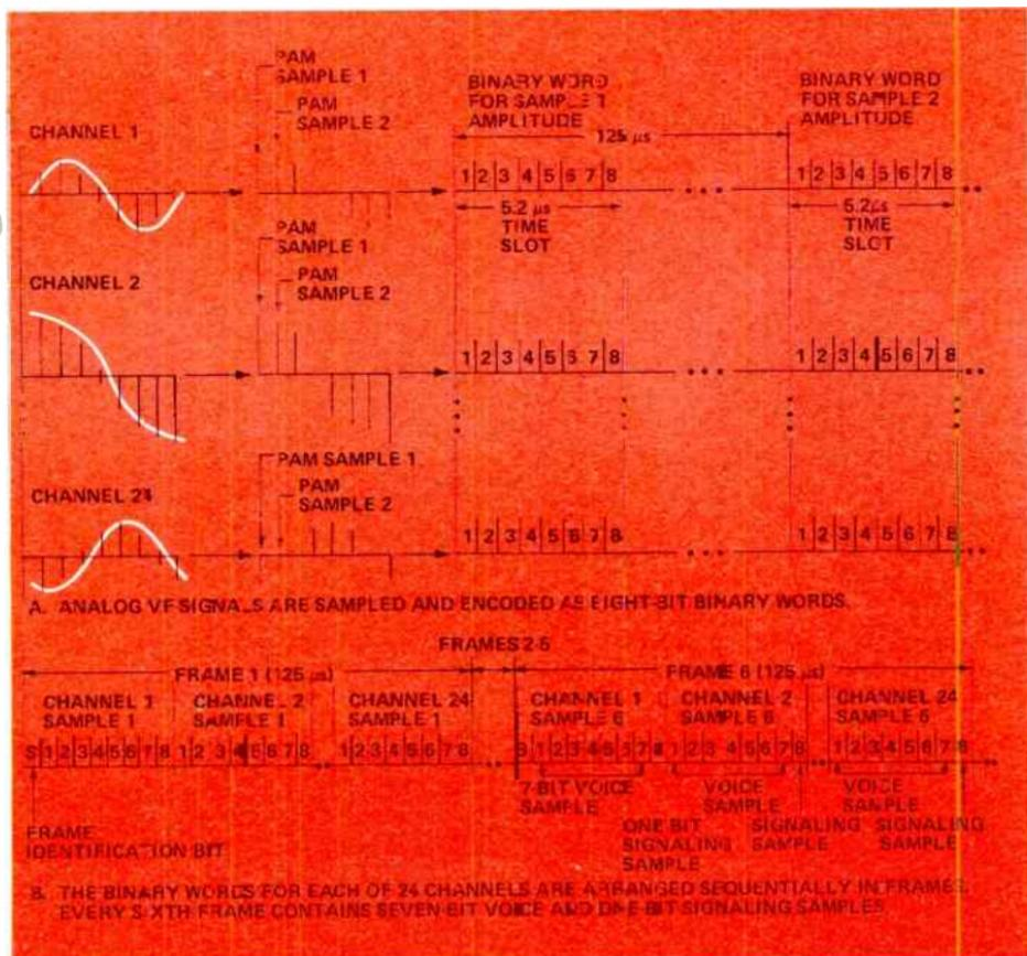
Figure 1. Basic encoding and organization pattern of signals in a 24-channel PCM transmission system.
