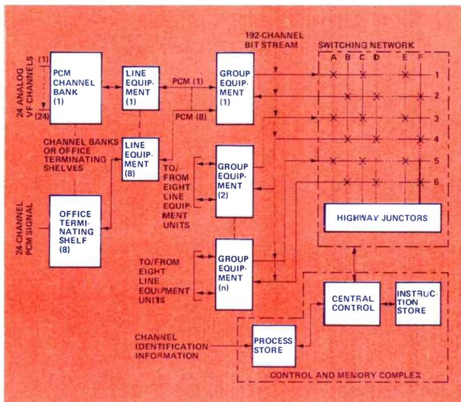
Figure 12. An electronic switching system in a space-time-space configuration.
