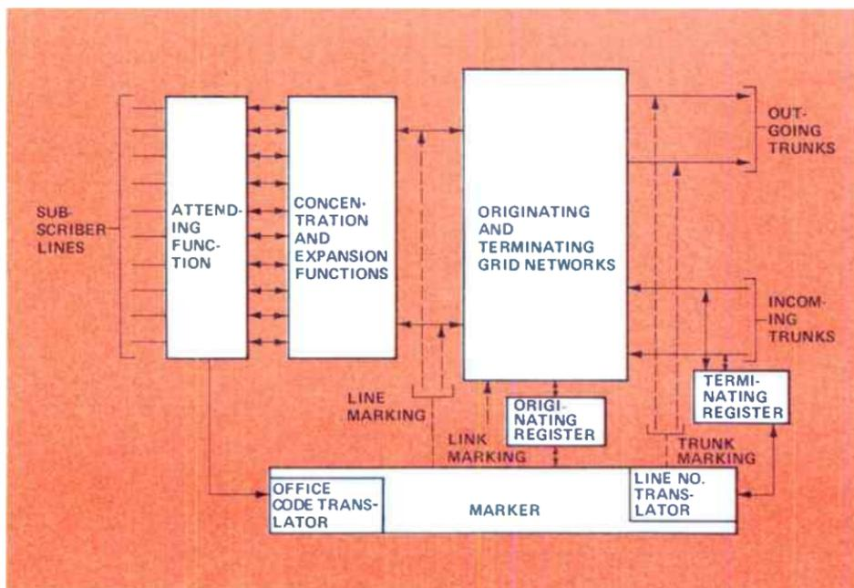
Figure 7. Combining functions in bidirectional networks allows common control techniques to be utilized in the most efficient manner.
