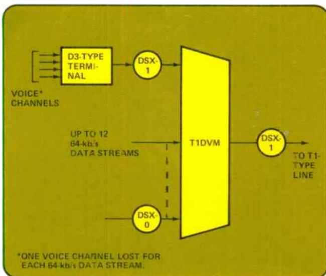
Figure 5. T1 Data-Voice Multiplexer (T1DVM) designed for low-density data routes permits substitution of 1 to 12 data streams for digitized voice signals.
