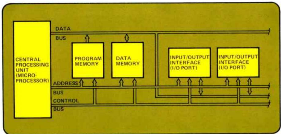
Figure 2. A microprocessor becomes useful only when it is associated with peripheral devices to form what is essentially a microcomputer.
