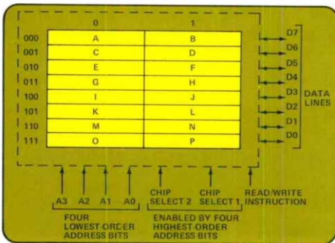
Figure 1. The unique address of each cell in a random access memory (RAM) structure allows the random recall or storage of data bits. In a read only memory (ROM) structure, data can only be recalled, but addressing is the same.
