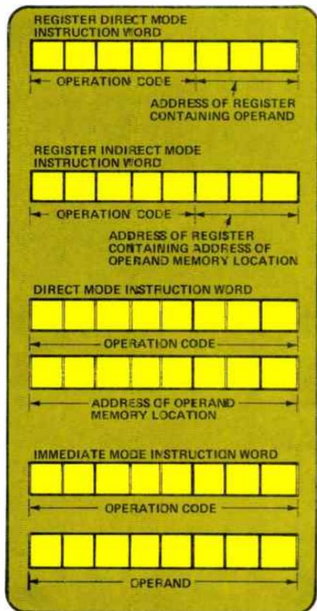
Figure 5. A microprocessor program may utilize several address modes to gain access to operands.
