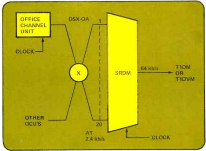
SRDM's can accept signals from OCU's operating at either 2.4 or 4.8 kb/s, and the 9.6-kb/s multiplexer can accept any of the three low-speed OCU signals, although there is a loss of efficiency when a submultiplexer is used at less than its maximum rate. All three versions of the digital submultiplexer have 64-kb/s outputs which connect to one port of a higher-order multiplexer.
