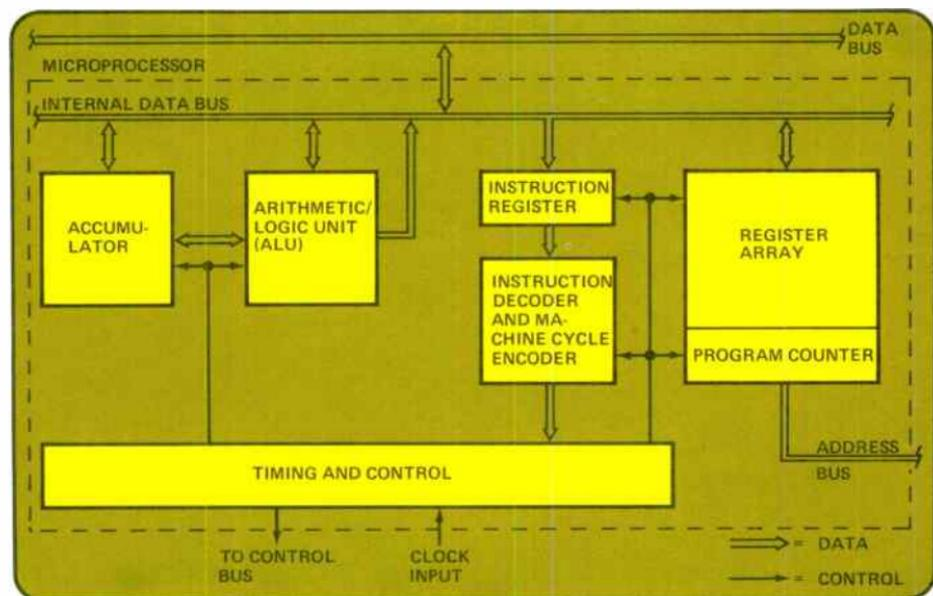
Figure 3. The structure of a microprocessor typically includes an arithmetic/logic unit, registers, and control circuitry.
