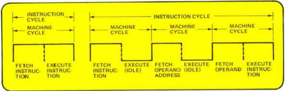
Figure 4. The instruction cycle of a microprocessor consists of one or more machine cycles, depending on the type of activity to be carried out.
