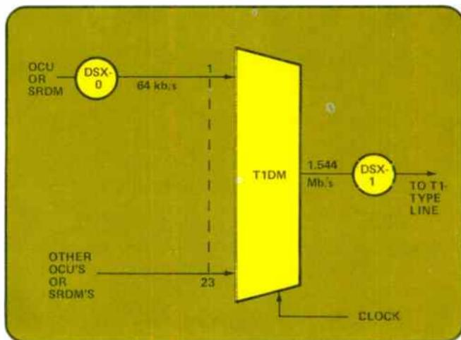
Figure 4. The T1 Digital Multiplexer (T1DM) designed for high-density data routes.
