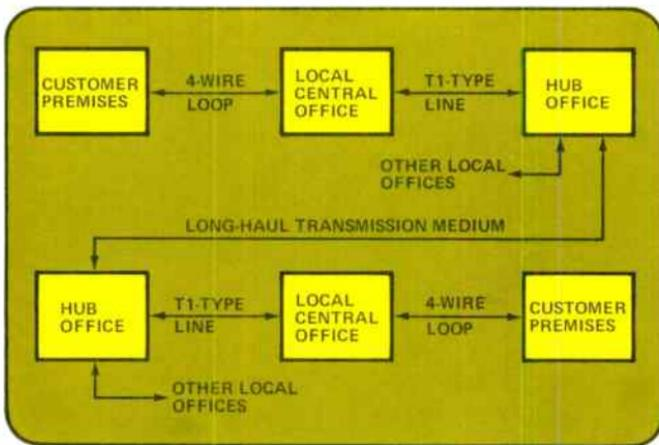
*Figure 1. Point-to-point DDS service provides an efficient path for data transmission without the need for cumbersome conversion equipment.*
