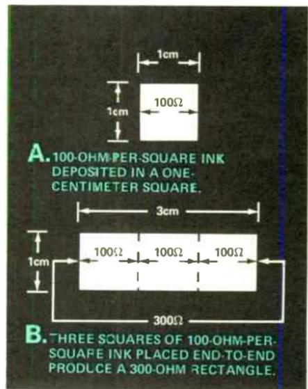
Figure 2. Thick film resistors are formed with special inks whose values are specified in "ohms per square."
