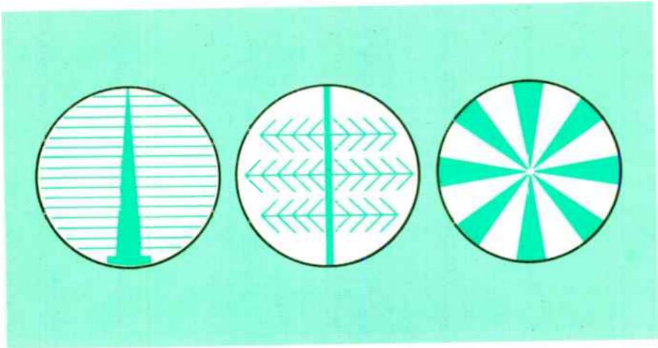
*Figure 1. These patterns are typical of collector grids which reduce the cell's series resistance. Square and rectangular cells usually have grids in finger-shaped patterns.*
