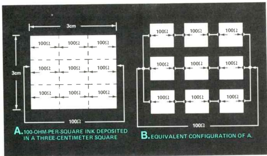
Figure 3. The resistance of a thick film resistor is a function of shape rather than size.
