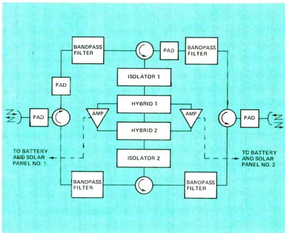
Figure 5. Simplicity of design and the elimination of the frequency conversion process permits the GTE Leukurt 700F1 RF Repeater to operate on less than four watts of power. Storage batteries provide 10-day backup capability for periods of prolonged darkness.
