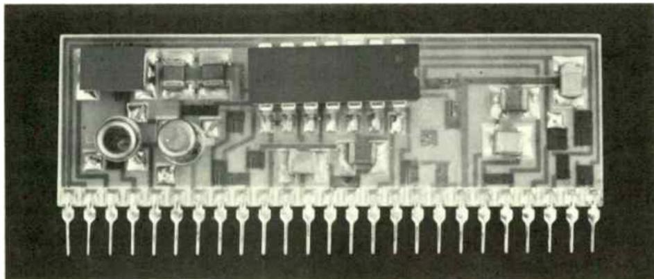
*Figure 1. Thick film hybrids combine discrete-component and monolithic technologies to produce circuits that retain many of the advantages of both.*
