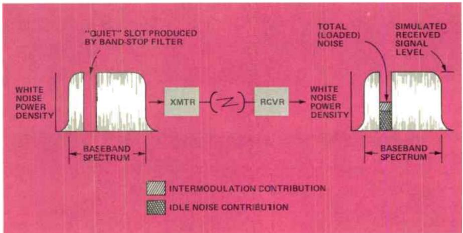
Figure 1. The loaded noise measured in a test slot is the product of both intermodulation and idle noise contributors. Depending upon the location of the slot in the spectrum and the characteristics of the contributors, the source of an impairment can be identified.
