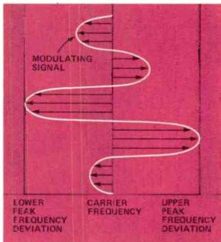
Figure 3. Changes of modulating signal amplitude produce deviation of carrier frequency.
