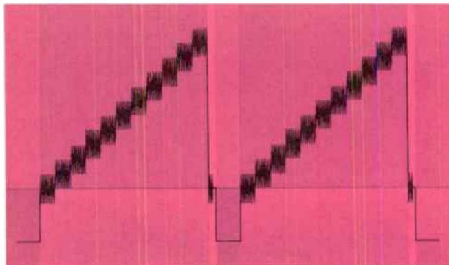
*Figure 6. Typical stairstep test signal, with simulated color subcarrier impressed, which can be used to detect nonlinearities, and to measure differential phase and gain, in a video system.*
