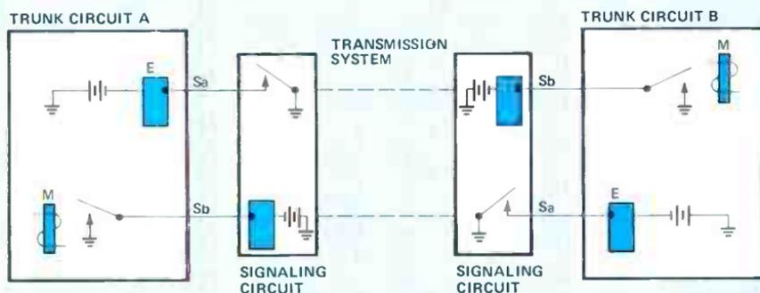
Figure 6. A representative international interface using F&M lead control. The Sa-Sb lead designations are typical of European products.
