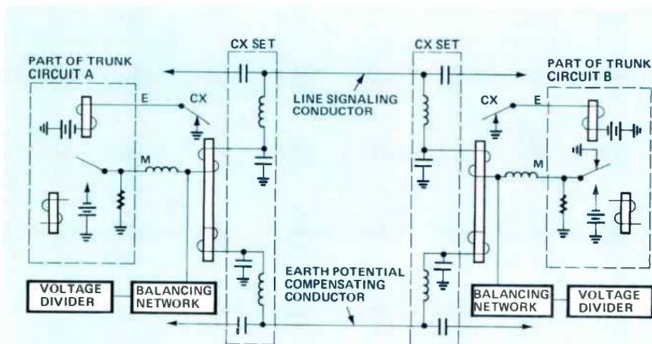
Figure 3. A composite signaling circuit with E&M lead control for one voice channel.
