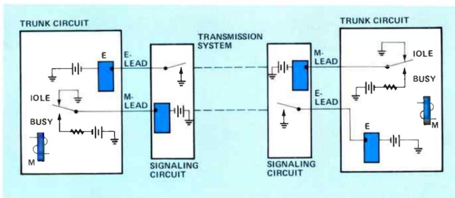
Figure 1. Traditional two-wire E&M interface (Type I) designed for electro-mechanical switches. Current between switching and signaling equipment returns over a common ground.
