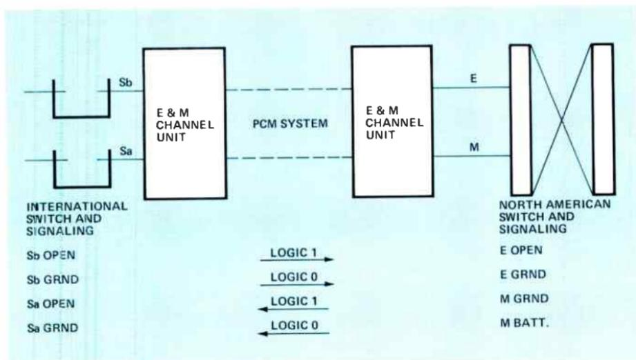
Figure 4. Block diagram of a North American switching and signaling system interfaced with an international type of system, both having E&M or equivalent leads.
