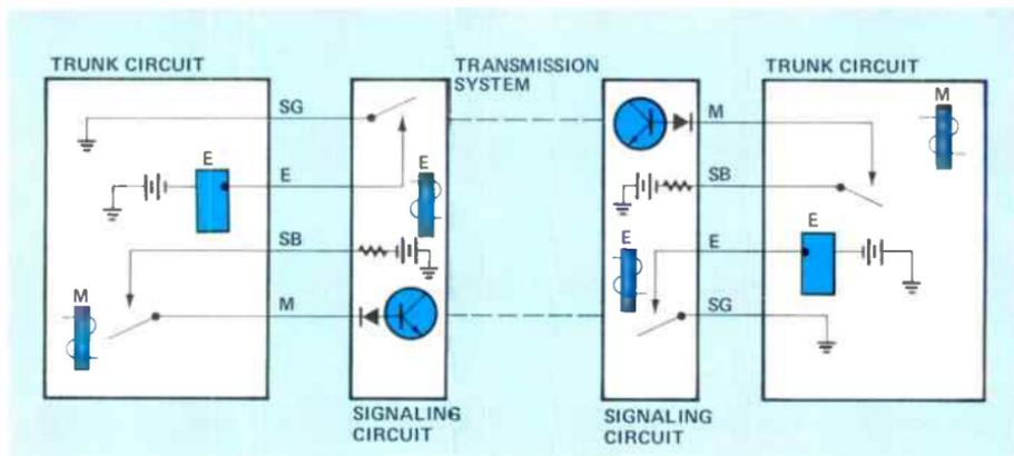
Figure 2. The Type II E&M interface for use with electronic switches has two leads for the M-signaling function.
