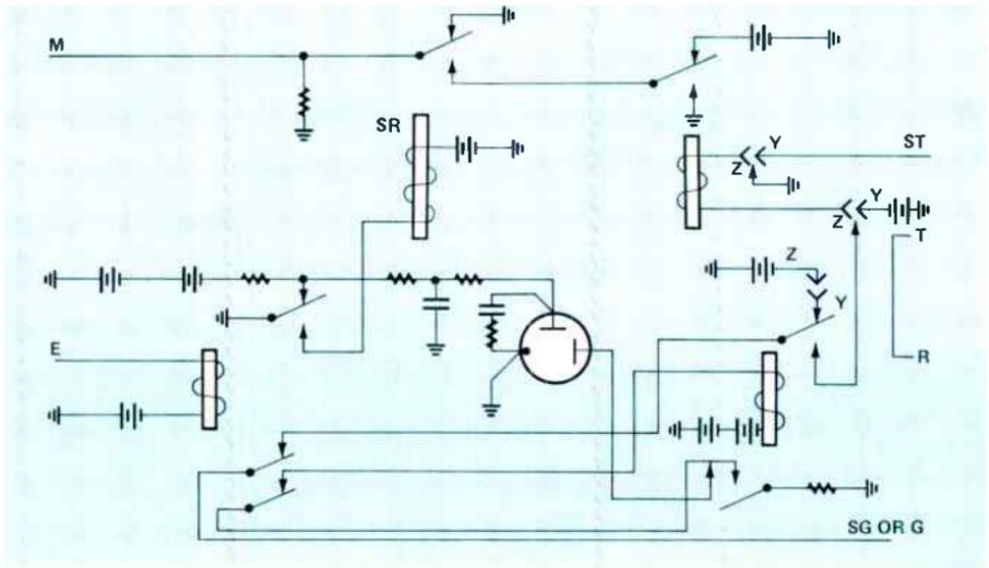
Figure 8. A typical ARI-type converter used with trunk circuits or signaling circuits equipped to receive 20-Hz signals.
