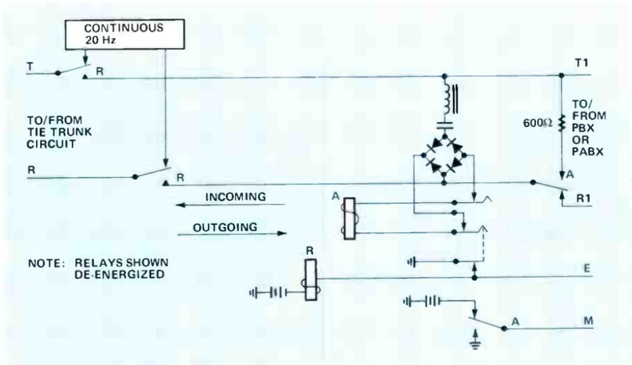
Figure 7. A typical converter used to convert from an SF or carrier section to 20-Hz, two-way ringdown operation.
