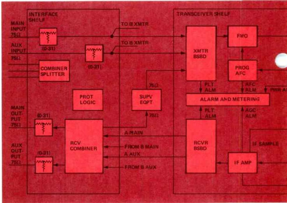
Figure 1. A typical hot-standby arrangement of the 2-GHz 79F1 radio is composed of an interface shelf, two transceiver shelves and an rf branching panel. The second transceiver shelf is not shown, but the interconnections between it, the interface shelf, and the rf branching panel are indicated.
