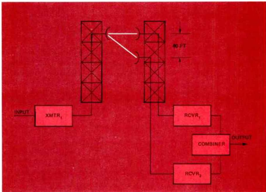
Figure 1. In a typical space diversity arrangement of a radio hop, the transmitted signal propagates over two separate paths to the receiving antennas.
