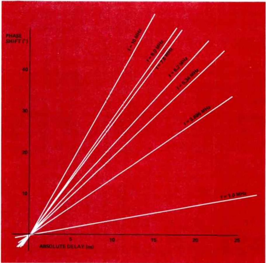
Figure 2. The phase shift between two signals increases linearly as the difference in their absolute delay and their frequency increase.
