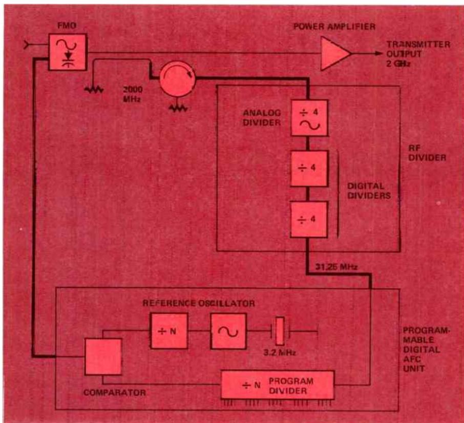
Figure 3. The new 2-GHz radio uses an rf divider instead of a reference oscillator, multiplier and mixer in the afc loop.
