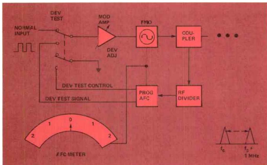
Figure 7. The deviation test circuit built into the transceiver shelf eliminates the need for external test equipment to set the deviation sensitivity of the radio.
