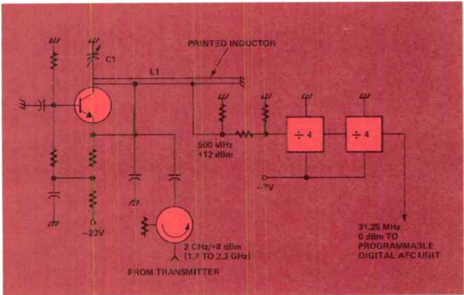
Figure 4. The injection-locked oscillator in the rf divider can be tuned by adjusting capacitor C1 to lock on any transmitter frequency in the 2-GHz band. The transmitter frequency is four times higher than the oscillator frequency.
