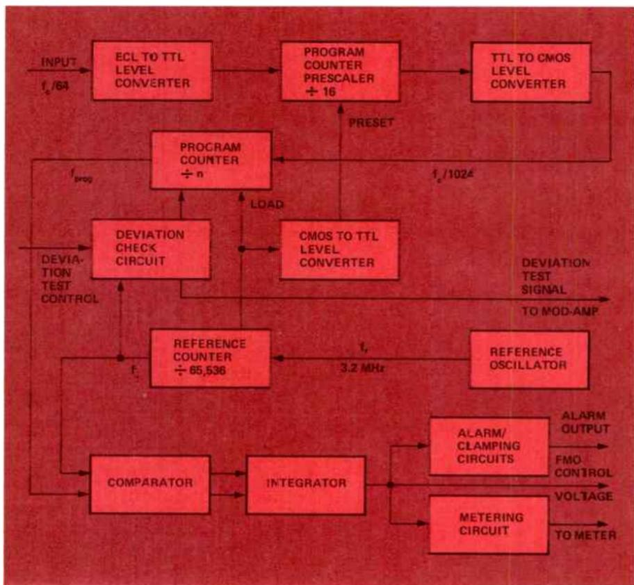
Figure 5. The primary function of the afc unit is to compare the divided frequency of the fmo to a very stable reference frequency and generate a dc control voltage proportional to the frequency error of the fmo.
