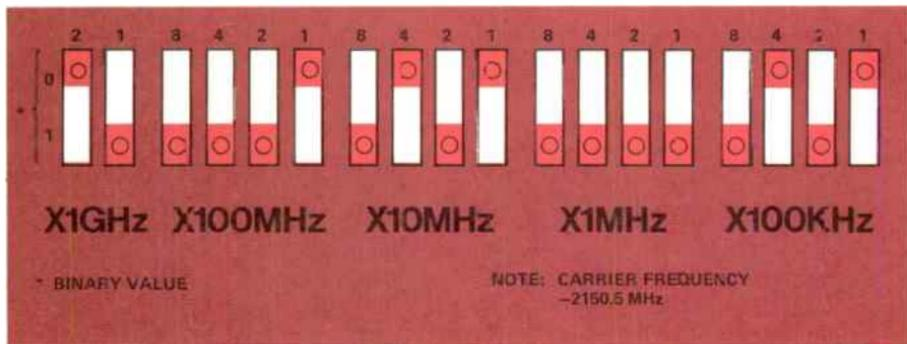
Figure 6. The positions of eighteen miniature strapping plugs are assigned binary values that represent the five most significant digits of the carrier frequency in binary-coded-decimal format. This is the program loaded into the program counter of the afc unit. The positions of the plugs in this figure represent a carrier frequency of 2150.5 MHz.
