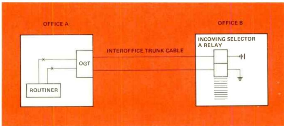
Figure 1. Outgoing Trunk Number Completing Test
