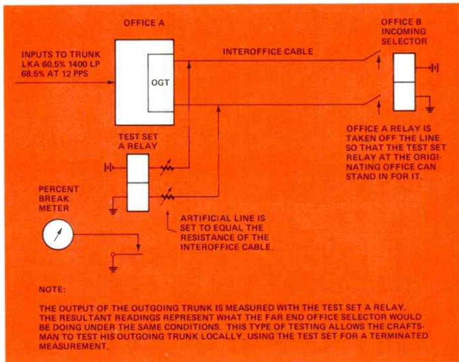
Figure 2. Local Pulse Repeating Test
