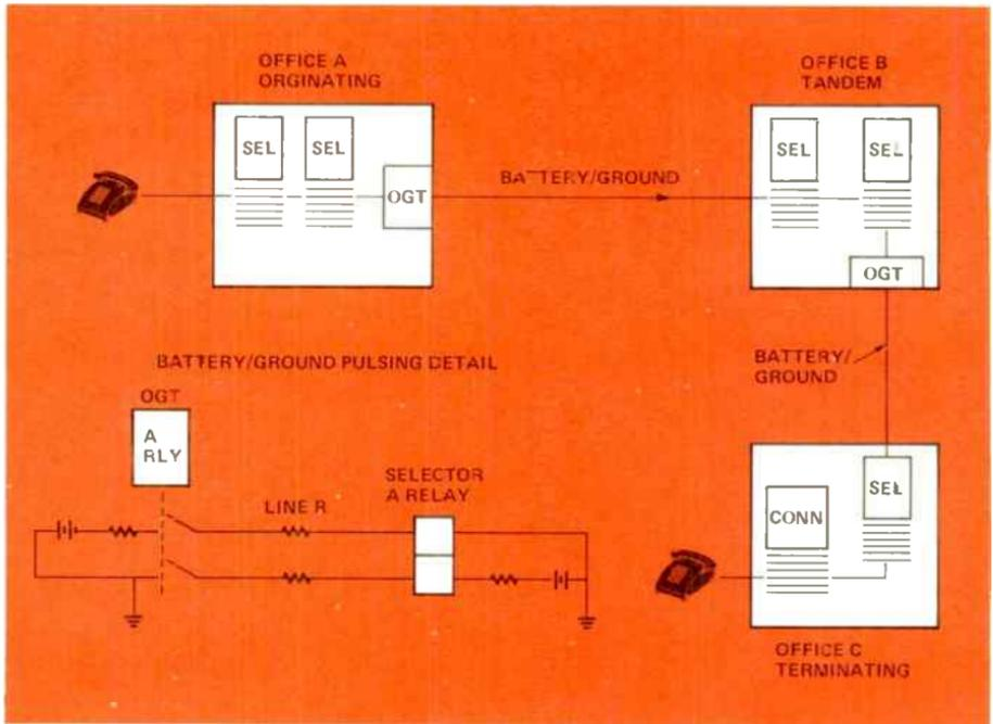
Figure 3. Tandem Physical Trunks
