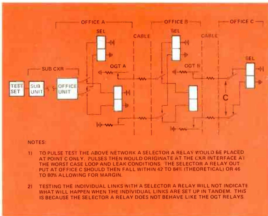
Figure 6. End to End Pulsing Test
