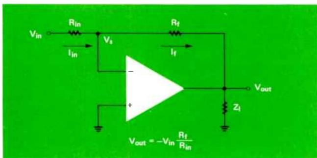
Figure 3. The voltage gain of the voltage inverter is determined by the ratio of feedback resistance to input resistance.
