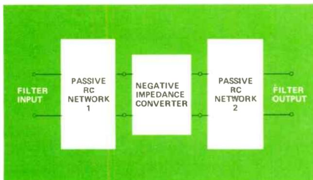
Figure 7. A negative impedance converter is typically placed between two passive RC networks to form a filter section.
