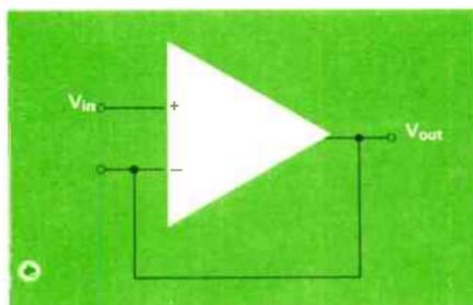
Figure 1. Voltage Follower. The name "Voltage Follower" is applied to this non-inverting operational amplifier because the output voltage is an exact replica of the input voltage.
