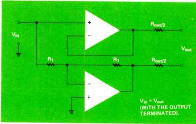
Figure 4. Unbalanced to Balanced Converter. This circuit is used where no gain is required. It uses a unity gain voltage follower buffer and an inverting amplifier.
