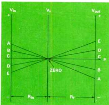
Figure 4. A graph of the electrical properties of the voltage inverter measured at certain points in the circuit at various instants demonstrates how current (slope of line) and output voltage vary with input voltage.
