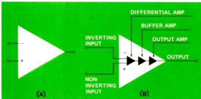
Figure 1. The schematic symbol generally used to represent an operational amplifier is a triangle with dual inputs and a single output (A). Most op amps consist of three direct-coupled amplifier stages (B).
