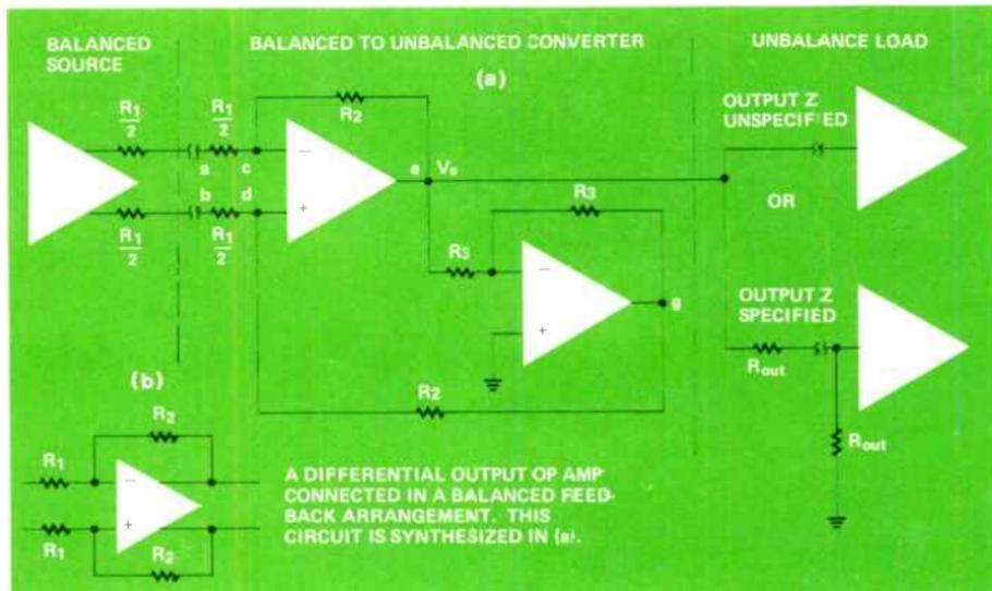
Figure 3. *Balanced to Unbalanced Converter. The circuit accepts a balanced input signal at a specified input impedance ( $R_{in}$ ) and converts it to an unbalanced signal with an unspecified output impedance or a specified impedance ( $R_{out}$ ).*
