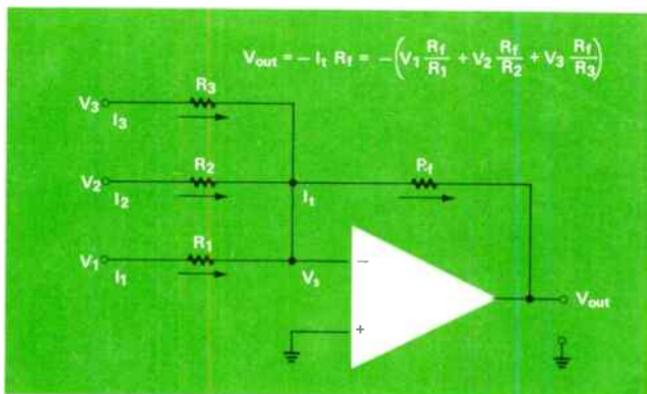
Figure 5. The summing amplifier circuit offers an electronic method for performing the mathematical operations of addition and subtraction.
