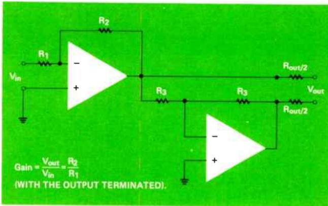
Figure 5. Unbalanced to Balanced Converter. This circuit is used when gain is required. It uses two inverting amplifiers.
