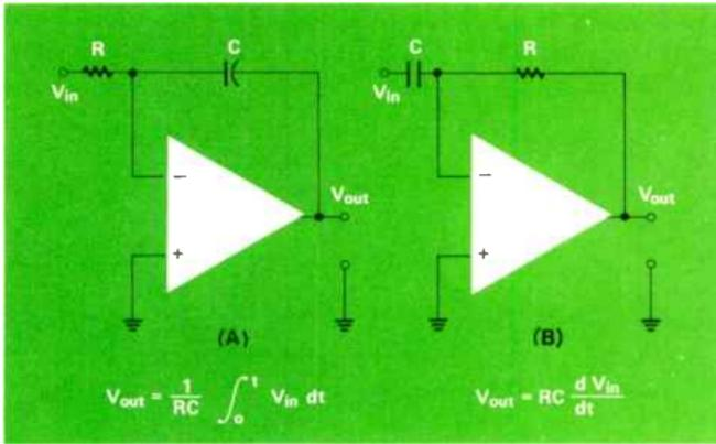
Figure 6. Inserting a capacitor into the feedback network in place of a resistor converts the inverting amplifier into an operational integrator (A) or operational differentiator (B).
