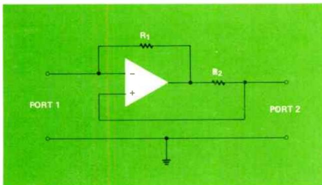
Figure 6. Realization of a current inverting negative impedance converter (INIC) using an operational amplifier.
