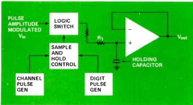
Figure 2. PCM sample and hold circuit. The holding capacitors must be quite small, so the amplifier input impedance must be very high to prevent capacitor discharge between pulses.
