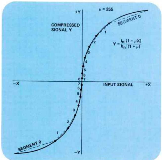
structured with 15 segments and 16 equal steps per segment, with step sizes in a ratio of 2:1 on adjacent segments and all step sizes an integral multiple of the smallest step, then the closest fit will cause  $\mu$  to equal 255.
