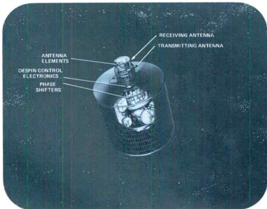
Figure 4. A cutaway drawing of the despun antenna system, initiated on Intelsat 3, shows placement of the phasers and radiating elements of the novel directional antenna developed by Sylvania Electronics Systems Division.
