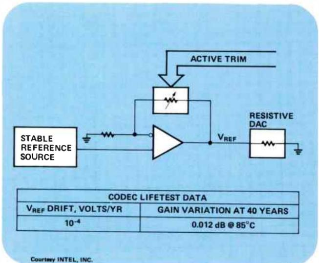
ence voltage equal to the difference. Flat band differencing is used to perform first order nulling of the temperature and voltage coefficients.
