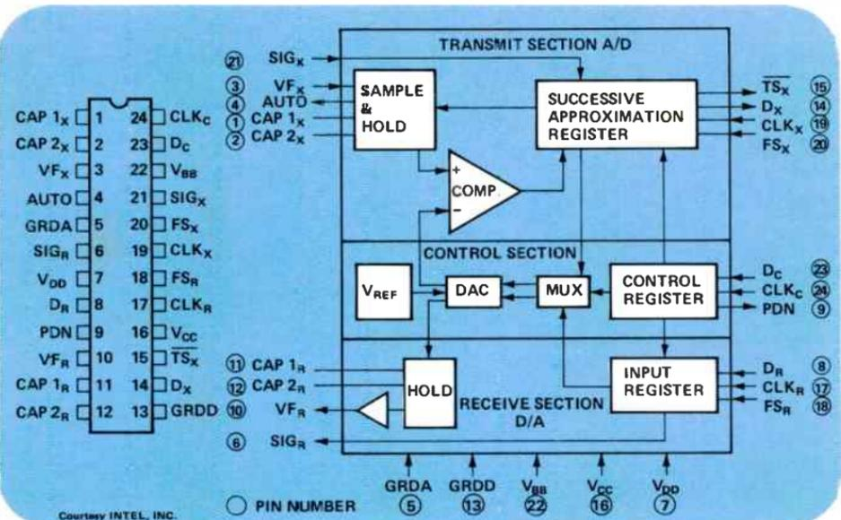
Figure 3. Pin configuration and block diagram for 2910 Codec.
