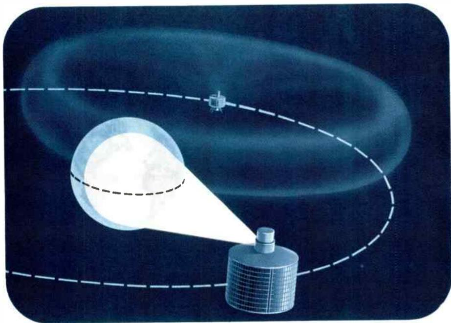
*Figure 3. Toroidal pattern of first communications satellites (rear) loses much rf energy in space. Intelsat III focuses its communications beam towards earth, using despun antennas with up to 16 dB gain.*
