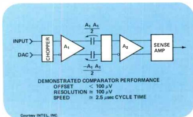
Figure 8. Low offset, high gain NMOS voltage comparator.
