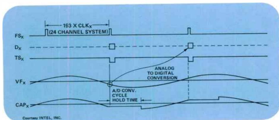
Figure 4. Analog to digital conversion.
