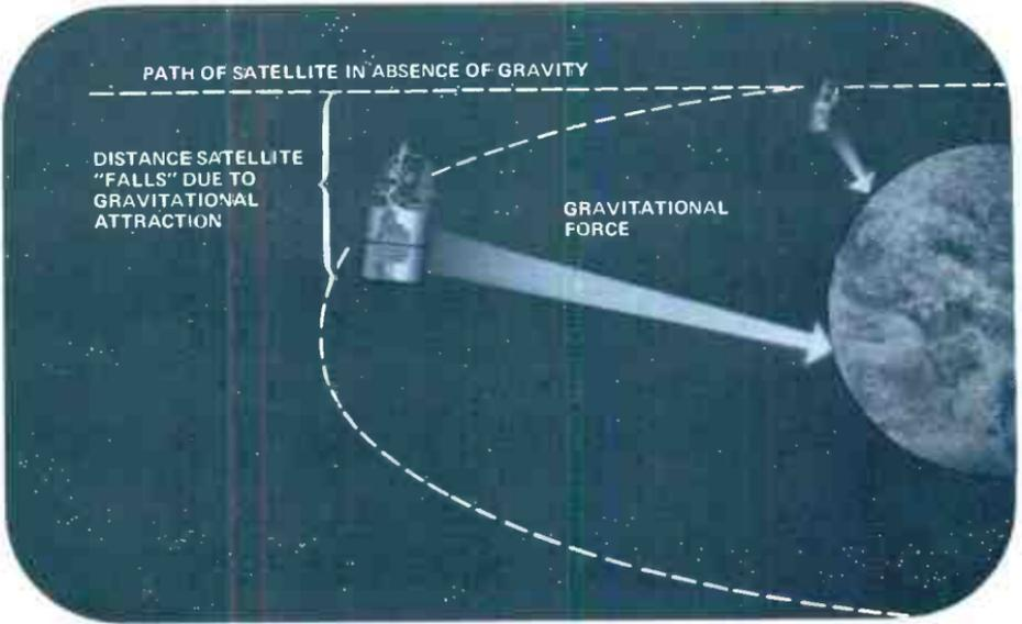
Figure 1. Tangential velocity of a satellite keeps it clear of earth, although it is constantly "falling" freely. When velocity, direction and gravitational field balance, satellite "falls" in a circular orbit. Because of small errors of speed or direction, most orbits are somewhat elliptical.
