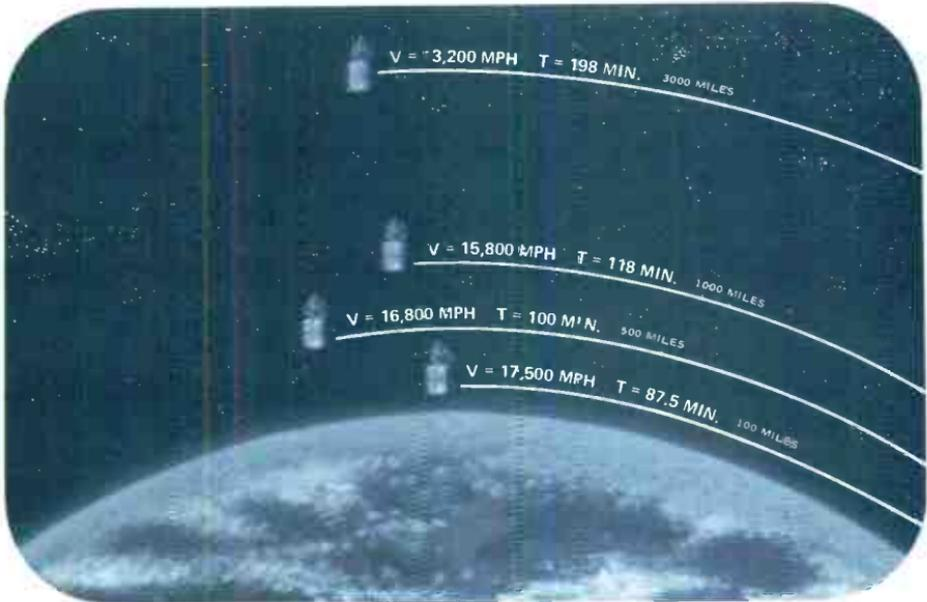
Figure 2. Gravitational force decreases with altitude, requiring lower velocities to maintain orbit. However, much more energy is required to drive the satellite to higher altitudes.
