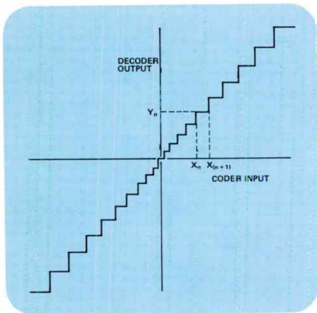
Figure 6. Non-uniform Codec transfer characteristic – more steps per volt for small samples than for large samples maintains a substantially constant S/D ratio.
