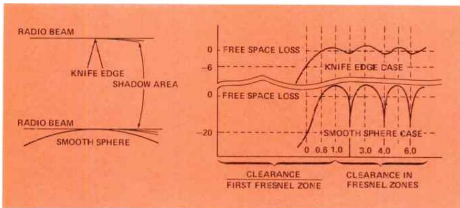
Figure 3. Diffractions caused by objects of different shapes.
