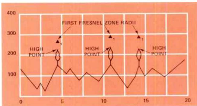
Figure 6. Fresnel zone clearance points.
