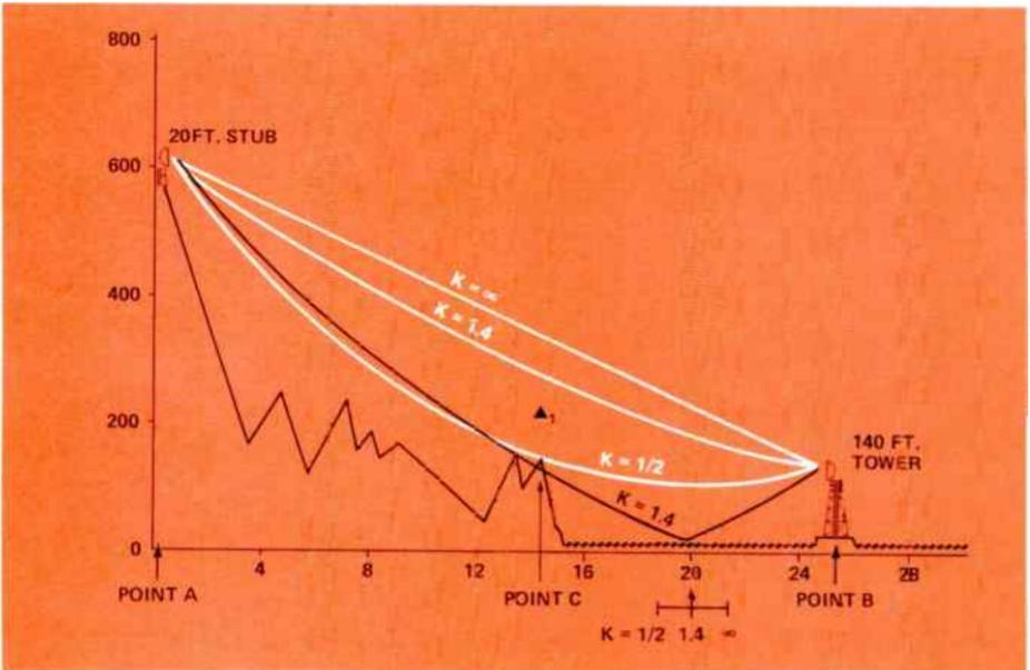
Figure 9. Obstructed reflection path.
