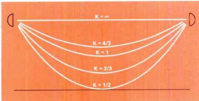
Figure 2. Relative beam curvatures for a flat earth.
