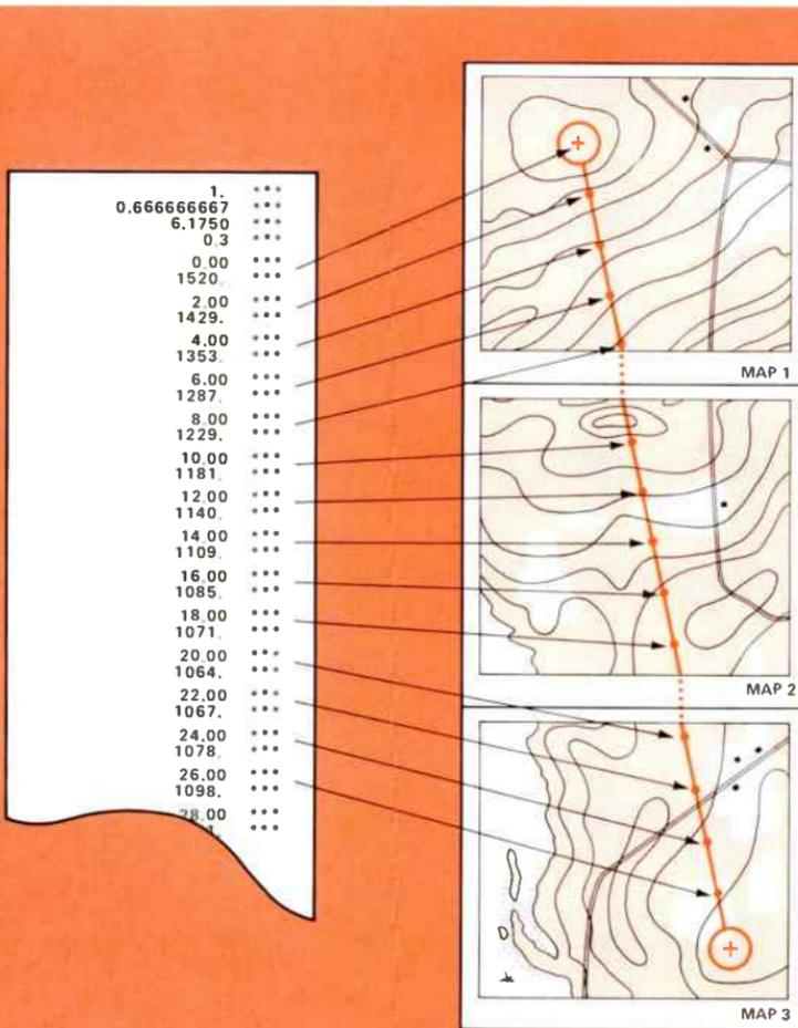
Figure 5. Checking map terrain against calculator generated output.
