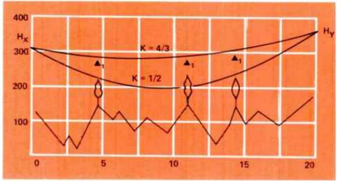
path, reflections can occur and affect the receive signal level. The Reflection Program can be used to calculate reflection points when the reflection point is level. Reflection points caused by sloping or rolling terrain can be adequately defined only by path tests.
