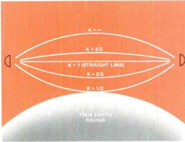
Figure 1. Beam refraction for true earth radius.
