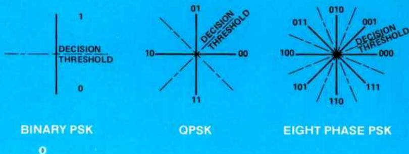
Figure 4. Relative phases and amplitude of PSK signals. The decision thresholds represent levels where the receiver must decide which signal has been received.
