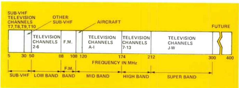
Figure 6. CATV Frequency Spectrum.
