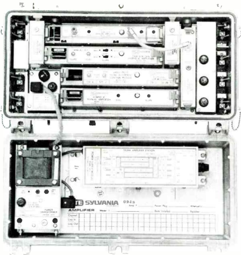
Figure 10. Trunk amplifier station.
