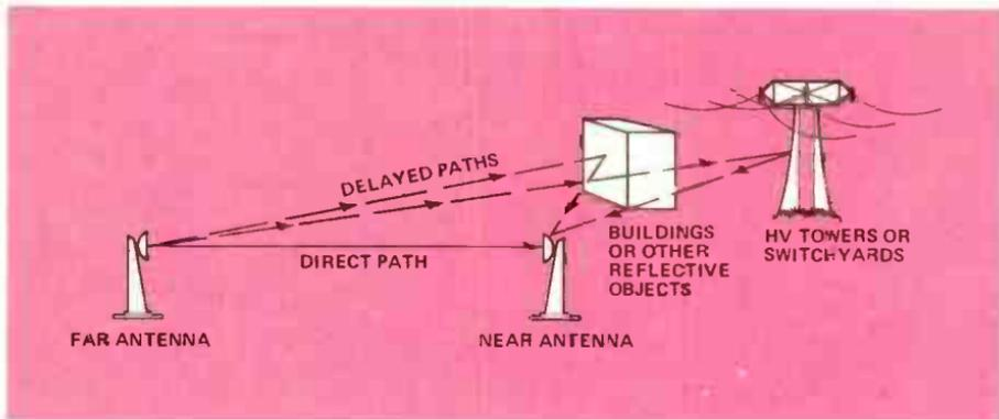
Figure 5. Rearward Multipath Distortion Mechanism (Correct by shrouding or raising the near antenna).
