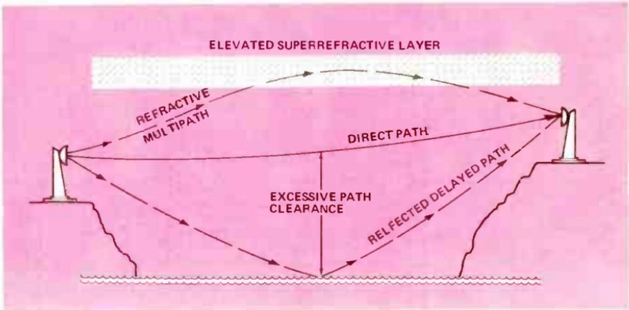
Figure 8. Multipath Distortion Caused by a Single Long-Delayed Reflected or Refracted Secondary Multipath Signal. Correct by Vertical Notching of the Lower Antenna For Minimum Distortion.
