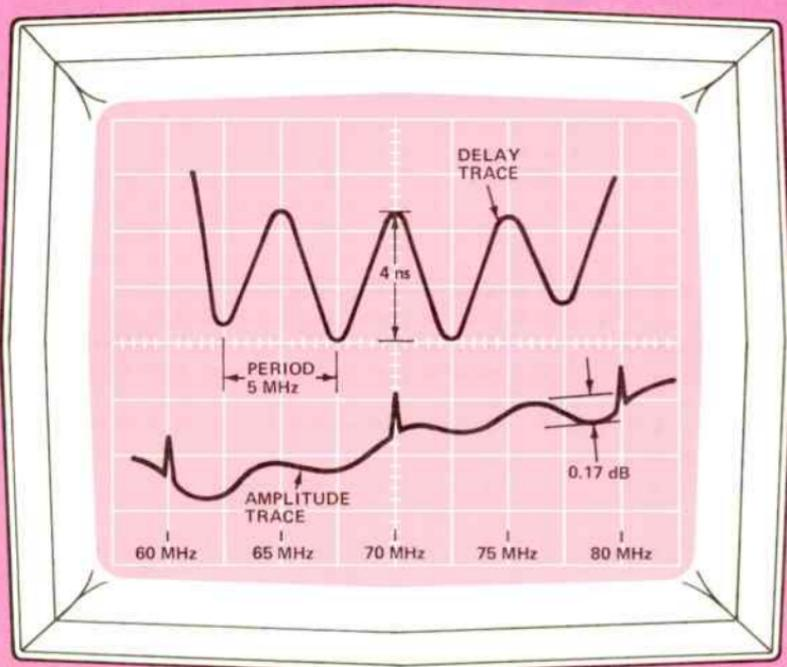
Figure 11. Artist's concept of a MLA IF Display showing a ripple caused by a multipath echo delayed 200 ns (196 ft. in free space) S/I = 40 dB.
