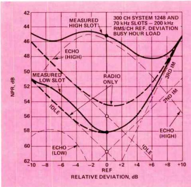
Figure 13. Bucket Curves showing high distortion due to a long-delayed (1000 ns) -38 dBm0 multipath echo. Note its influence in the low slot.
