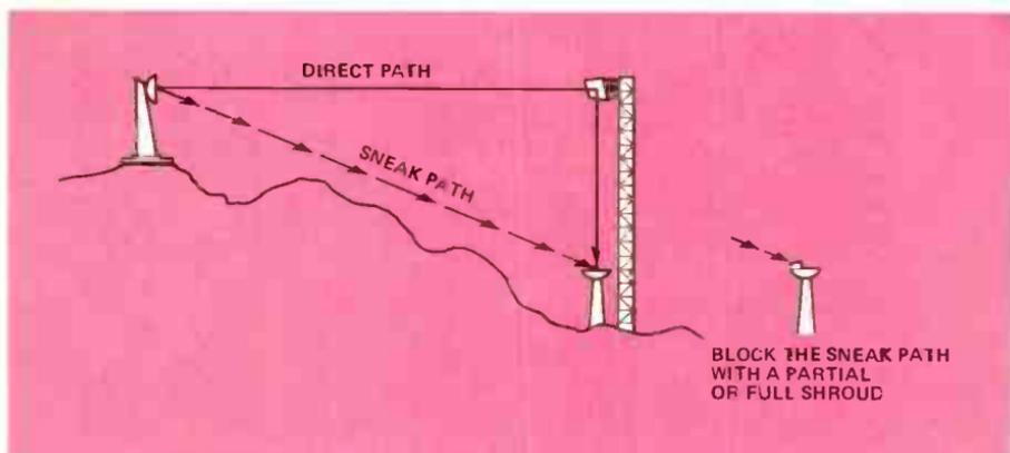
Figure 7. Periscope Antenna Multipath Distortion Mechanism.
