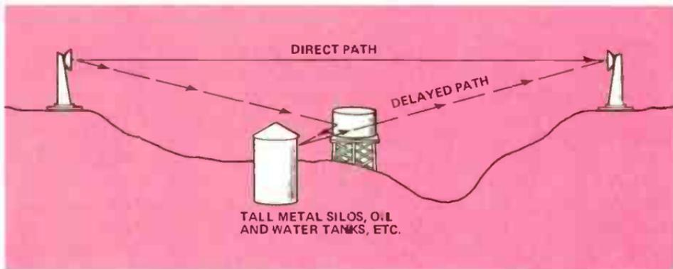
Figure 2. On-Path Double Reflection Mechanism (Often not correctable except to minimize direct path fading — see figure 1)
