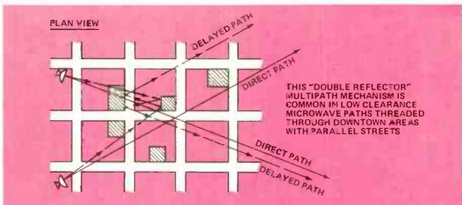
Figure 6. Metropolitan Area Multipath Mechanism. Parallel building walls generate an on-path echo signal irrespective of path azimuth.
