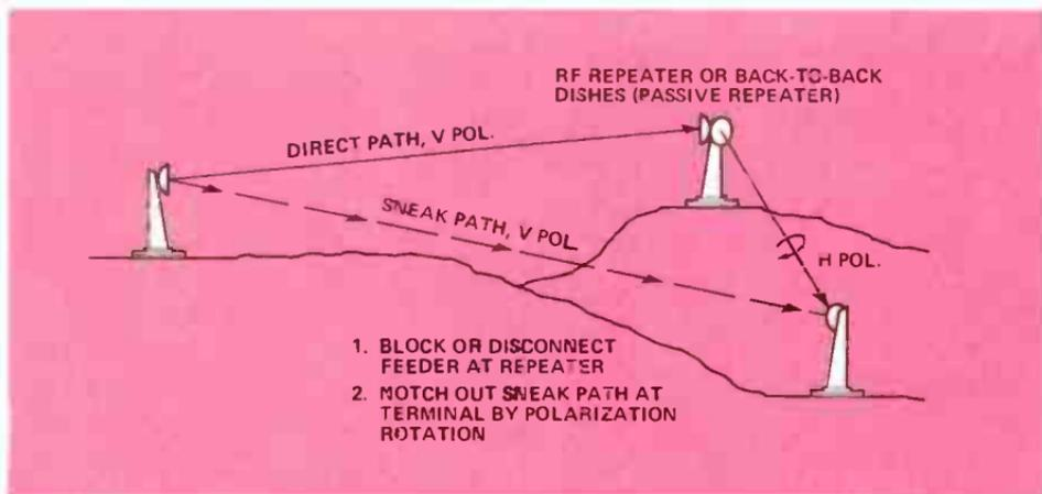
Figure 3. Multipath Distortion in Back-to-Back Passive or RF Repeaters.
