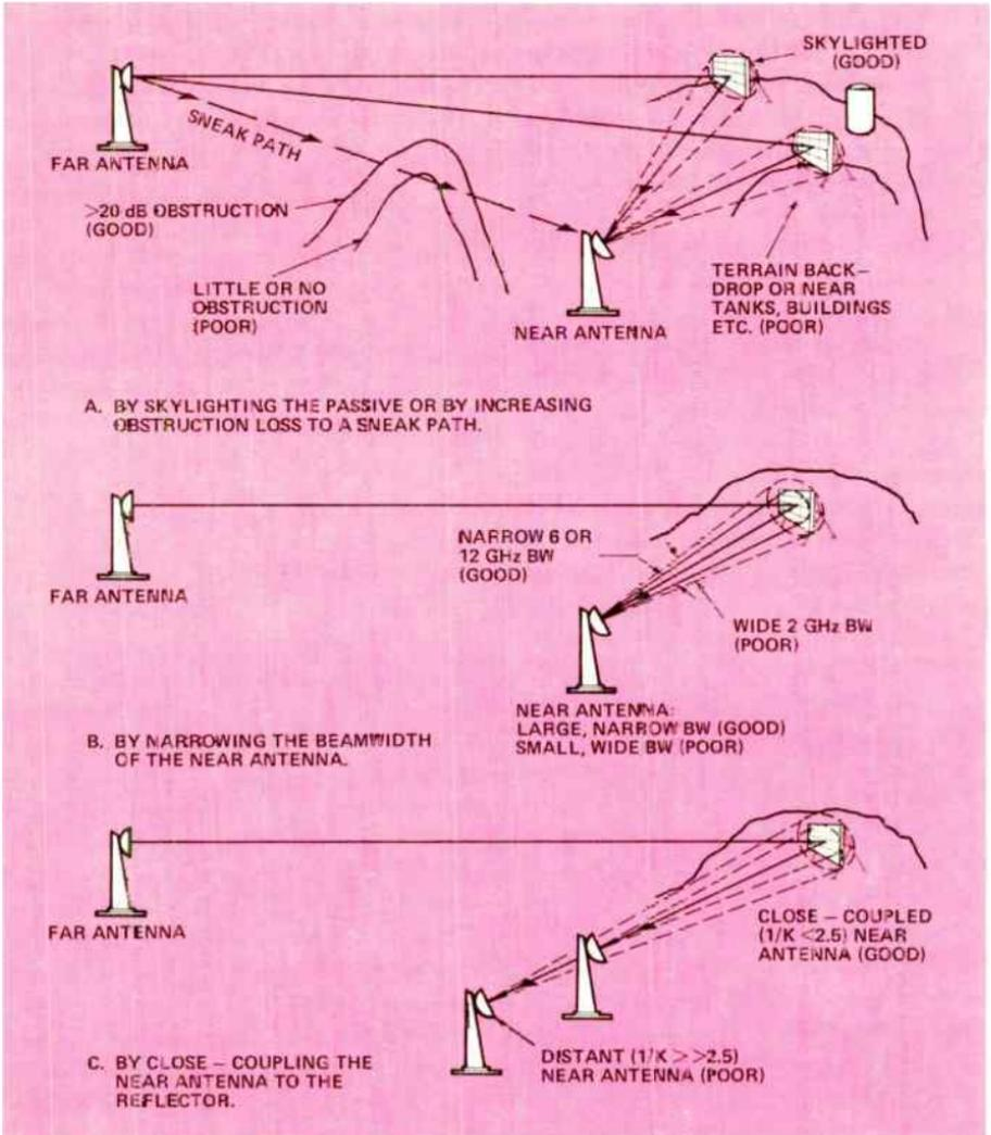
Figure 10. Methods of Reducing Multipath Distortion in Passive Reflector Systems (After near-end antenna notching).
