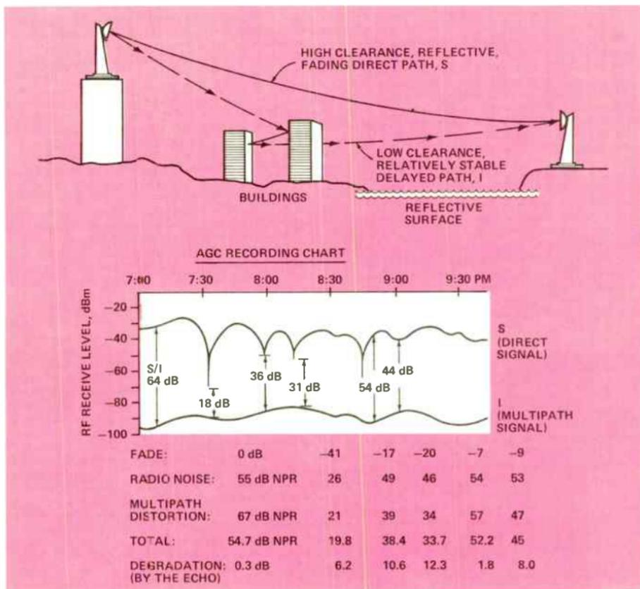
Figure 1. Multipath Distortion in a Fading Environment (Delayed multipath/direct signal fades are uncorrelated). Correct by minimizing direct path fading or by raising or increasing the size of the close-in antenna.
