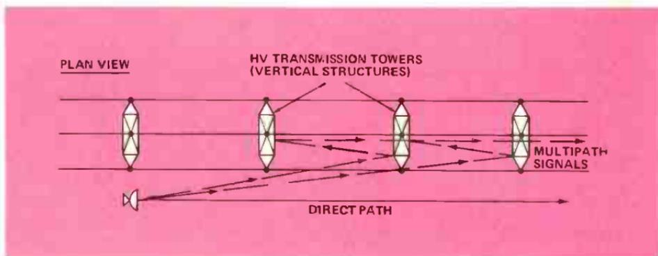
Figure 4. Multipath Generated When a Microwave Path Parallels (and is close to) A HV Transmission Line Supported by Vertically — Faced Towers. Correct by horizontal antenna notching or larger antenna.
