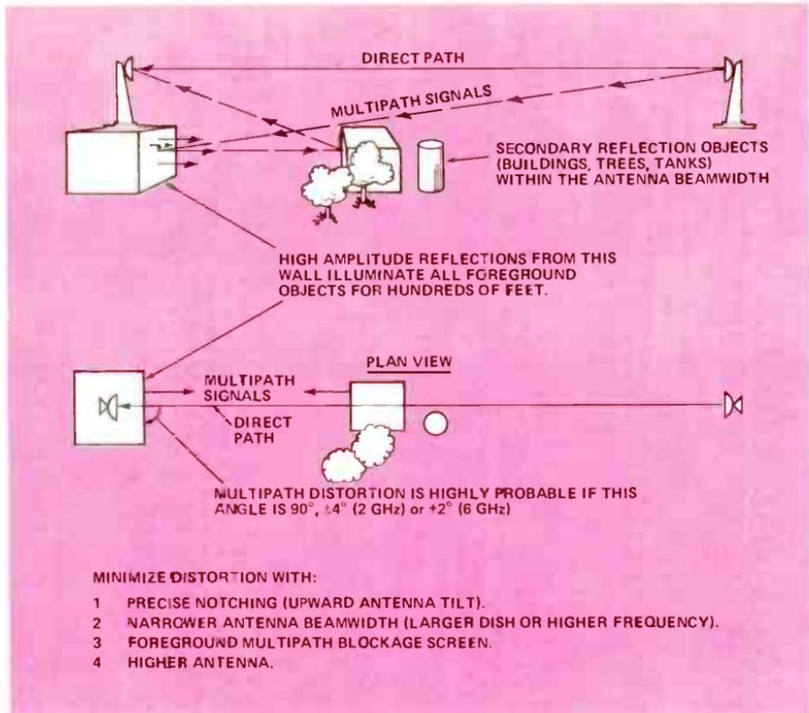
Figure 9. The "Floodlamp" Multipath Distortion Mechanism.
