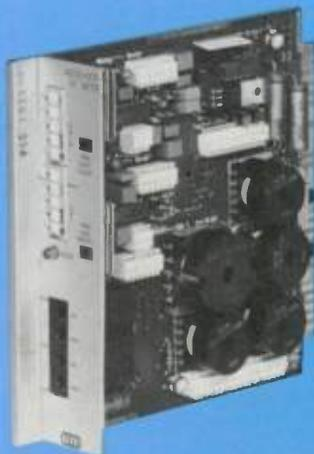
The 4600 VFR is a four coil hybrid repeater with front panel, prescription gain and equalization. The 4600 operates with positive net loss (gain) in most applications.
