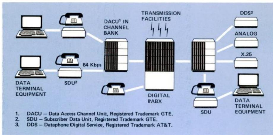
Figure 2. Star Topology — Second Generation PBX digital switching. Data is accommodated through data ports. Some intelligence is in the terminals.
