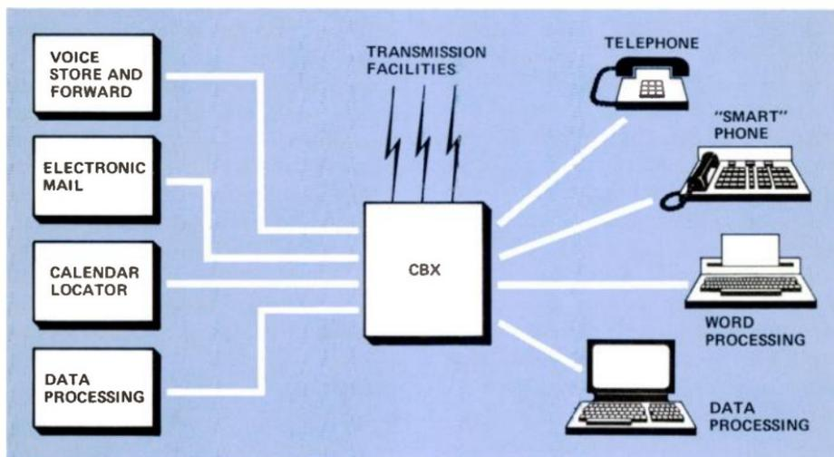
Figure 3. Star Topology — Third Generation PBX. The CBX functions primarily as a switch to connect the user with specialized processors as well as data processors. Speed, code and protocol conversions may also be provided depending on the computer's capacity. Some intelligence is in the terminals.
