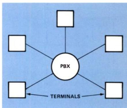
*Figure 1. Star Topology — First Generation PBX. The PBX acts as a switch. There is no requirement for intelligence in the terminals.*
