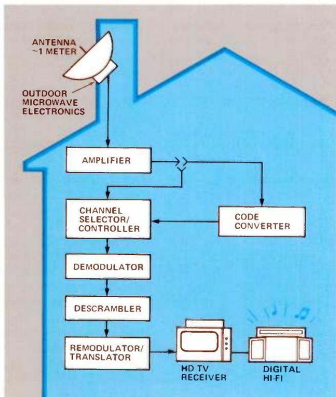
*Figure 2. Direct Broadcast Satellite Home Receiver For High Definition TV.*
