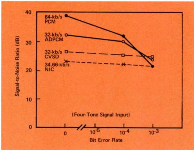
Figure 7. Objective Signal-to-Noise Ratio as a Function of Bit Error Rate.
