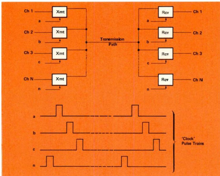
Figure 3. Diagram of a Simple TDM System.
