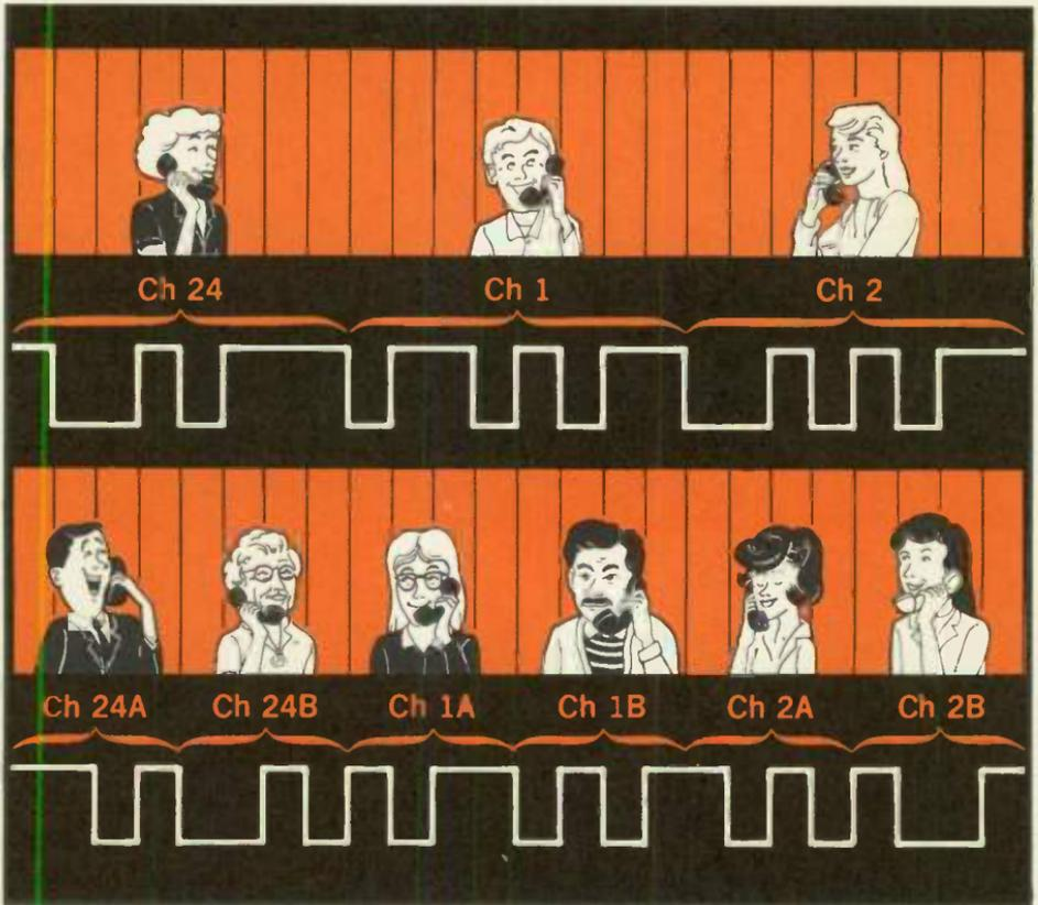
Today, pulse code modulation (PCM) common carrier telephone systems use a 64-kb/s encoding scheme for each voice channel. However, a substantial amount of research is underway to develop schemes that use an encoding rate considerably less than 64 kb/s per channel. The advantage of a lower bit rate is that more voice channels can be carried by a given transmission system, considering its digital rate or bandwidth.
