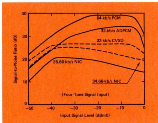
Figure 6. Objective Signal-to-Noise Ratio.
