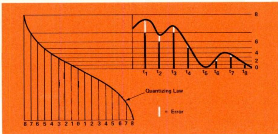
Figure 4. Changing a Linear to a Non-Linear Quantizing Scale.
