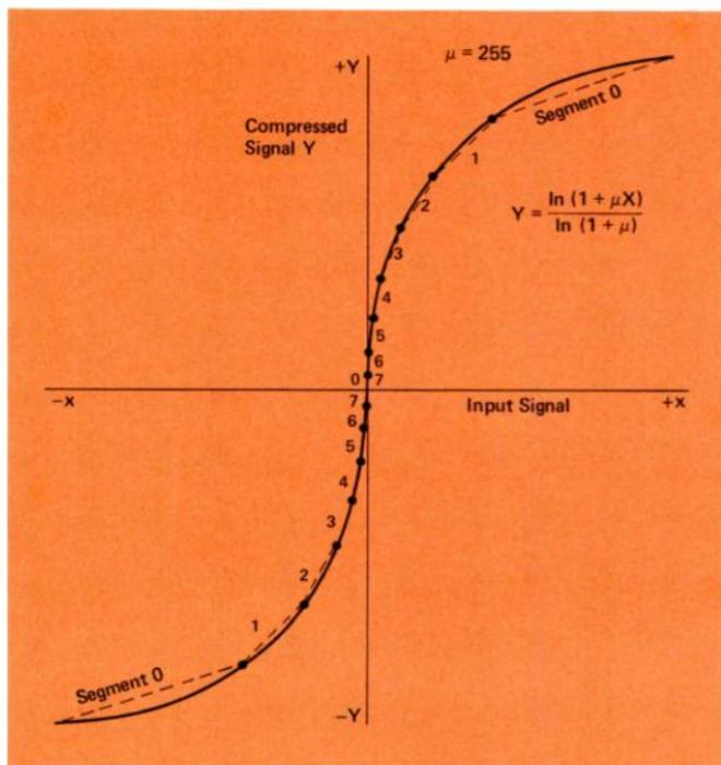
Figure 5. Segmented Compression Characteristic.
