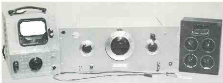
FIGURE 1. This voltmeter, oscillator, and decade resistance box are typical of the instruments that can be used for measuring transmission line characteristics.
