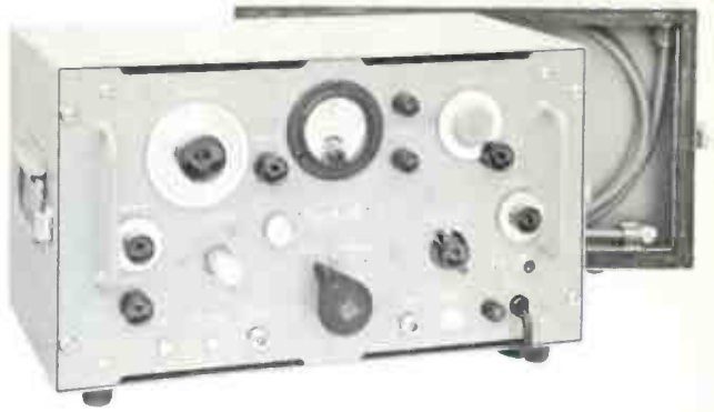
Fig. 1. A typical test set for measuring power and frequency on waveguide circuits.
