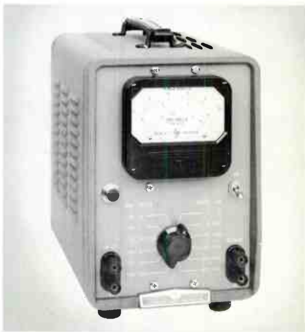
Fig. 3. Hewlett-Packard type 400D vacuum tube voltmeter. This meter has a flat frequency response from 10 cps to 4 mc. Input impedance is in excess of 10 megohms so that when connected across 500,000 ohms or less, there is negligible effect on the circuit being tested.
