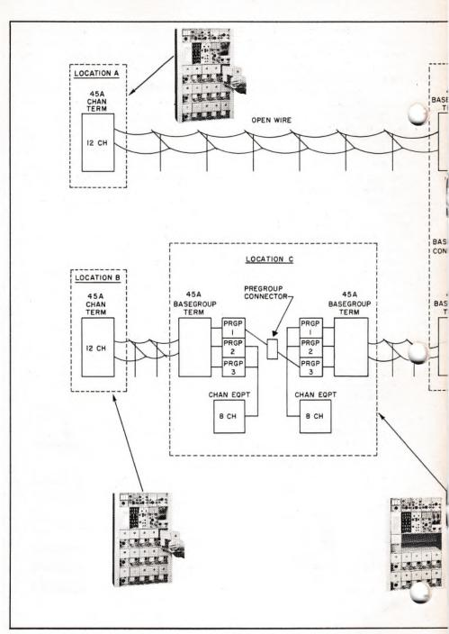
FIGURE 2. Typical 45-class carrier network. A 12-channel basegroup is transmitted from station A to station F over three different transmission media. Basegroup transfers are made at the junctions of the media at stations D and E. Similarly, an 8-channel group (2 pregroups) is transmitted from station C to station F, being
