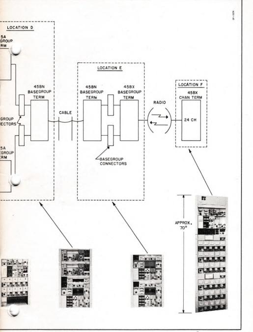
combined with the 12-channel group at station D. From station B, a 4-channel pregroup is transmitted to station F with a pregroup transfer being made at station C. The 45A system between stations B and C is also used to provide 8-channels directly between these two points. The photographs show the actual equipment (less compandors) required at each station.
