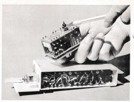
FIGURE 1. Experimental model of a transistorized, print wired, line amplifier compared to equivalent vacuum tube type. Pointer indicates transistor raised above its normal position.
