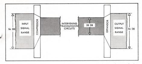
FIGURE 2. Compression and expansion of various signal intensities in a typical compandor for telephone applications. The compressor is at a -16 db level point. The expandor is at a +7 db level point.
