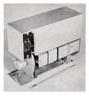
FIG. 2. Directional Filter Unit. This unit is shown strapped to transmit the 60-76 kc band and receive the 40-56 kc band.
