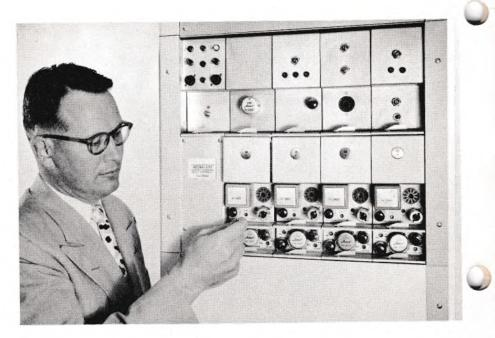
FIG. 1. A complete 4-channel terminal assembly of Type 45CB carrier equipment. This assembly occupies only 15-3/4 inches of vertical rack space.
