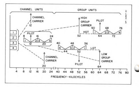
FIG. 6. The frequency allocation and modulation plan of Type 45CB carrier.
