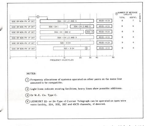
FIG. 1. Additional circuits which can be derived from an open-wire pair with Lenkurt's 33A and 45CB Carrier Systems.
