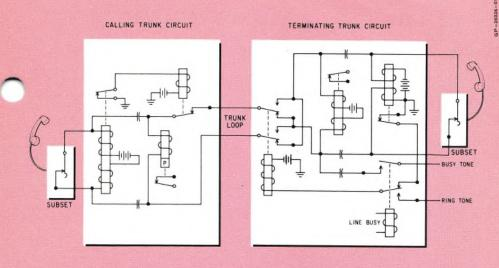
Figure 2. Typical reverse battery loop supervision circuit. Only supervisory relays are shown.
