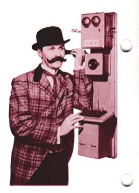
Figure 1. First automatic telephone employed both magneto and push-button signaling for establishing desired connection.
