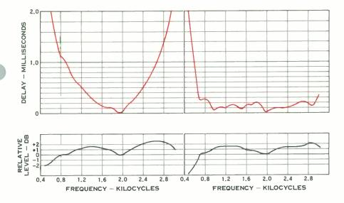
Figure 3. Amplitude and delay characteristics of a cable carrier channel before and after equalizing delay. In this 450-mile path, signal was translated down to voice frequencies four times.
