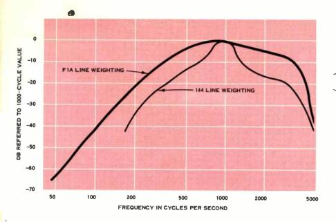
Figure 4. Weighting curves show the relative interfering effect of noise on speech when using either Type 144 or F1A handsets or their equivalents. F1A curve is international standard.
