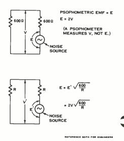
Figure 5. Psophometric noise is measured or calculated in volts (or millivolts) under conditions shown here.
