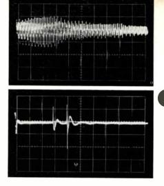
Figure 2. Comparison of speech and noise impulse recorded from actual telephone circuit. Speech sample is the word "two." Note slight ringing following each noise impulse.
