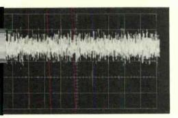
Figure 1. "White" noise as it appears in communication channel. Other names for white noise include background noise, random noise, and fluctuation noise.
