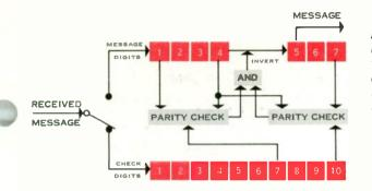
Figure 6. Decoder for burst-correcting code. Twenty error-free digits are required between bursts to "recharge" check digit register, thus imposing severe limitation on this type of code.
