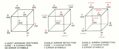
Figure 4. Solid geometry allows mathematicians easy way to analyze effciency and other characteristics of complicated codes. Simple 3-digit example shown requires three-dimensional figure. Each vertex represents a code combination assignable to characters or errors.
