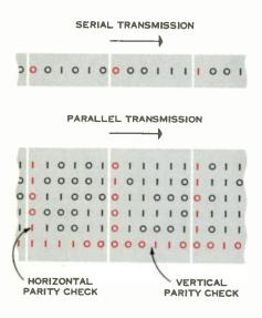
Figure 3. Typical parity checks for serial and parallel transmission. Check digit is chosen so that sum of marks in each block of data is always even (odd, in some codes). Error is revealed if wrong count is received. Compensating double errors may go undetected. can be detected. A third parity check added for the remaining digits will further reduce the undetectable errors.
