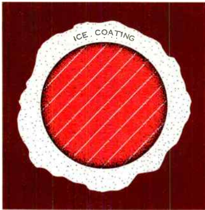
Figure 4. Current flow in a conductor covered with ice. Dot distribution indicates density of current flow.
