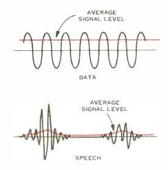
Figure 5. Data signals flow continuously and evenly into a voice channel, while the flow of speech is sporadic. Thus data has a much higher average level than speech and imposes more severe loads on multichannel amplifiers.
