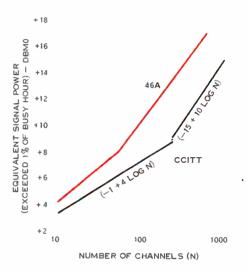
Figure 6. A comparison of the loadhandling characteristics recommended by the CCITT and the characteristics of the Lenkurt 46A. The 46A will carry substantially more data traffic than allowed for in CCITT recommendations.
