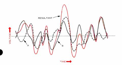
Figure 4. Phase addition of two random speech signals (A and B). High voltage peaks appear in the resultant whenever the individual signals peak together.
