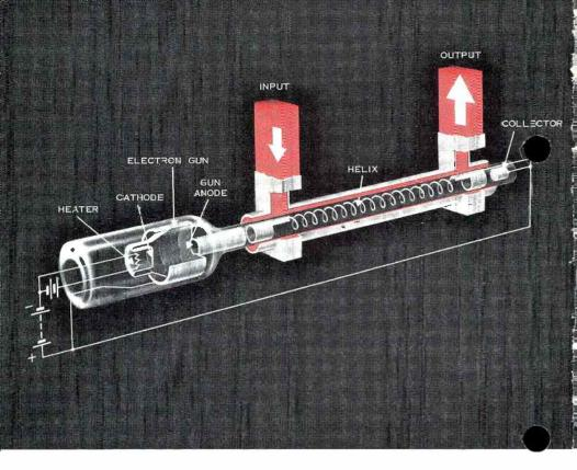
Figure 1. Construction of a typical traveling wave tube, showing the electron gun, the helix, and the collector.
