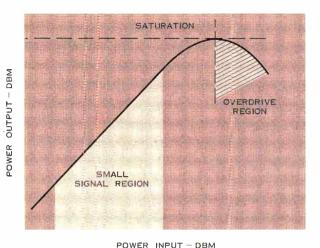
Figure 5. Power output vs. power input.
