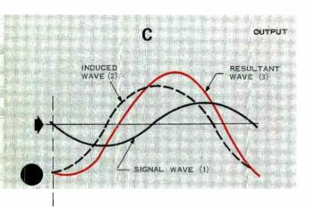
Figure 3. As the signal wave travels down the tube, electron bunches induce a second wave on the helix. The resultant of the signal wave and the growing induced wave increases exponentially.
