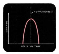
Figure 6. Gain vs. helix voltage.
