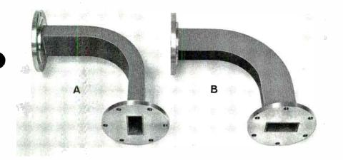
Figure 3. Two types of 90° bends for rectangular waveguide. Because the bend of waveguide A is in the plane of the electric field, it is referred to as an E bend. Waveguide B is referred to as an H bend because the bend is in the plane of the magnetic field.
