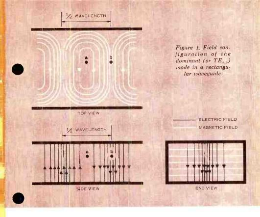
of propagation. This class of modes is known as the TE or *transverse electric* class. In the second class of modes, the magnetic field is always perpendicular to the direction of propagation. This class is known as the TM or *transverse* magnetic class. The two fields are mutually perpendicular to each other and oriented at right angles to the direction of propagation.
