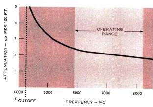
Figure 2. Attenuation versus frequency characteristics for a typical rectangular waveguide.
