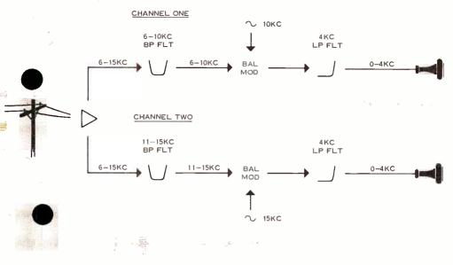
Figure 3. Simplified two-channel telephone multiplex system.
