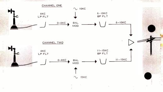
rection of transmission. This permitted the use of filters to separate the channels and the hybrid coils were no longer necessary. This technique of using different frequencies for each direction provided what is known as an *equivalent 4-wire* system.
