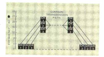
Figure 1. In frequency division multiplexing, low-frequency speech signals, ranging between 0 and 4 kc, are shifted to separate positions in a higher frequency range.
