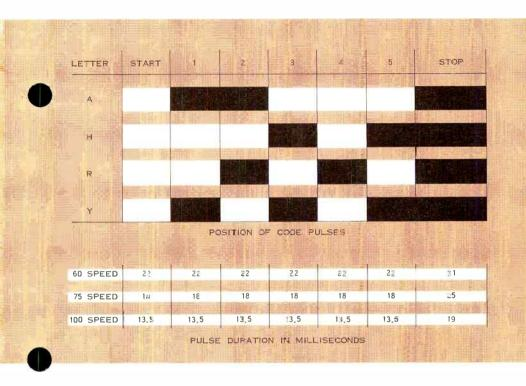
Figure 1. Examples of the 5-level Baudot code for the letters A, H. R, and Y. including pulse lengths for the three standard telegraph speeds. Mark pulses are shown in color while space pulses are shown in white.
