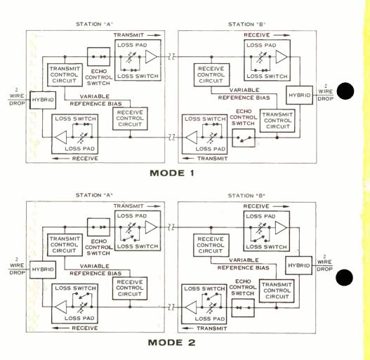
Figure 4. Simplified diagram of Mode 1 (uni-directional) and Mode 2 (bidirectional) operation of the Lenkurt 931B Echo Suppressor.
