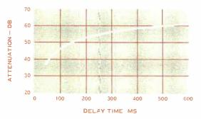
Figure 3. The attenuation needed to suppress echoes to tolerable levels is indicated for the average telephone talker.
