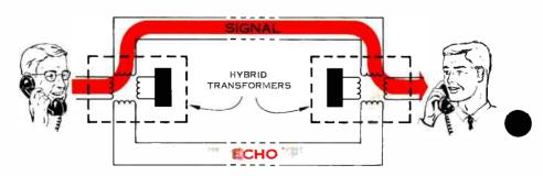
Figure 2. Hybrid transformers are needed at each end of a 4-wire circuit. Reflected energy at this point becomes echo.
