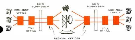
Telephone path through exchange, toll and regional offices. Echo Figure 1. suppressor is located at the beginning of 4-wire toll circuits.
