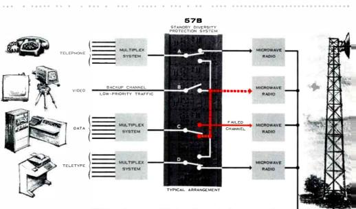
**Lenkurt's 57B and 57C systems** provide standby protection economically for large microwave systems, where many radio channels link the same locations. The 57B system provides one-for-three standby protection using baseband switching, while the 57C system provides two-for-six standby protection using IF switching. Both systems are capable of protecting microwave radio systems handling up to 1200 message channels or one TV signal.
