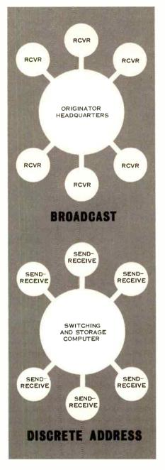
Figure 1. Data communications systems fall into one of two general categories. One is essentially a receive-only system while the other has stations with a send and receive capability.
