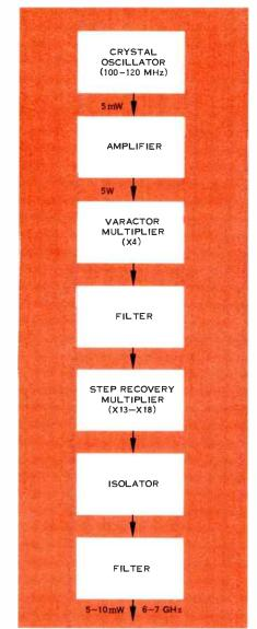
Figure 1. Typical solid-state local oscillator design uses crystal oscillator frequency reference source, varactor diode multiplier for times four multiplication and step recovery diode for times thirteen to times eighteen multiplication. Microwave frequency in the 6 to 7 GHz range, determined by the step recovery multiplication, has from 5 to 10 milliwatts output.
