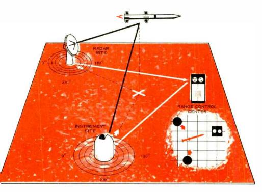
Figure 3. Radar picks up missile after launch, sends polar coordinate tracking information to the range control center. Computer translates to Cartesian system, sending pointing information to other instrument sites.
