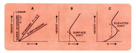
Figure 3. Typical M profiles showing atmospheric conditions. Profiles B and C indicate an inversion which can cause ducting. Each profile has associated with it different propagation characteristics.
