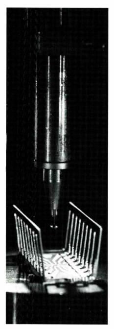
Figure 6. Recently developed technique shows Fairchild integrated circuit about to be mounted face down on frame. All contacts are made at one time.
