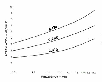
Figure 3. Response curves compare the attenuation versus frequency characteristics of the common types of communications coaxial cable.
