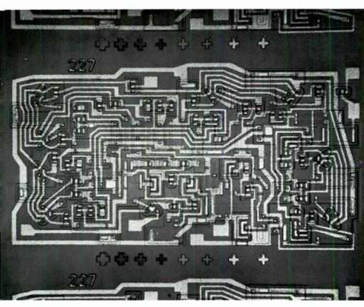
Figure 7. Sylvania IC contains 116 transistors, resistors and diodes to produce 40 gate circuits on each chip. Used in computers or digital communications equipment.
