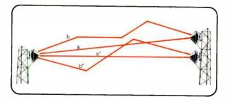
Figure 7. With space diversity the same wavelengths travel different refracted paths (b and b') but will not have the same interfering effect on the direct waves (a and a').
