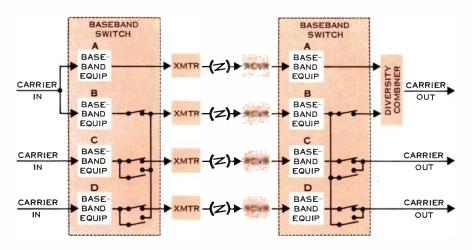
Figure 8. Block diagram of typical standby diversity protection system. Channel B operates in frequency diversity with channel A, while providing backup for channels C and D in the event of a failure.
