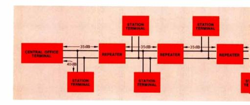
kHz. Up to three repeaters may be added at approximately the 20 to 40 dB loss points along the cable. Repeaters extend the maximum length out to 140 dB.
