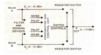
Figure 7. Simplified diagram of typical combination equal-gain optimalswitching combiner circuit.
