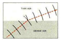
Figure 1. The velocity of microwaves traveling through the atmosphere increases as the refractive index of the air decreases. The increased velocities at the top of the wavefront cause the microwave beam to bend.
