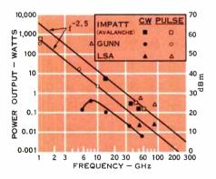
Figure 1. Maximum power produced by three solid-state devices. Note that the maximum pulsed power of the IMPATT avalanche type diode and Gunn diode decreases as frequency increases in the proportion  $f^{-\varepsilon.s}$ .
