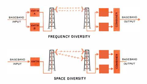
Figure 4. Two types of diversity reception commonly used in line-of-sight microwave systems are frequency diversity and space diversity.
