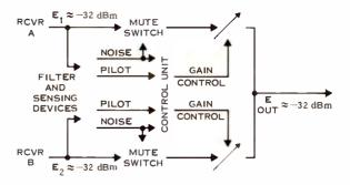
Figure 6. Simplified diagram of typical variable gain combiner circuit.
