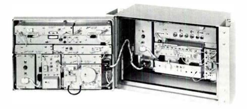
Figure 3. Construction of the Lenkurt 71F 2-GHz Microwave Radio typifies the advanced modular design and high density packaging afforded by total solid-state construction.
