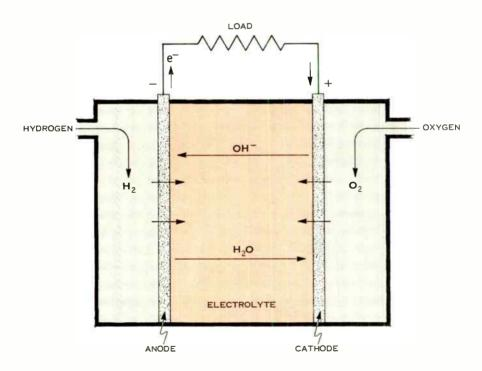
Figure 2. At the anode of the hydrogen-oxygen fuel cell. hydrogen joins with hydroxl ions to produce water, freeing electrons to do work. At the cathode, oxygen reacts with water in the electrolyte and electrons from the external circuit to form hydroxl ions.
