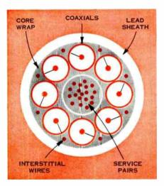
Figure 1. Typical communications coaxial cable consists of a number of "pipes" or "tubes" together with interstitial wires and service pairs inside a single sheath. Each pipe or tube provides one-way transmission for a large number of message channels or a TV signal.
