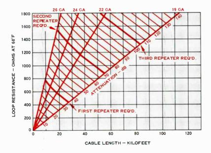
Figure 3. Cable design chart for 82A station carrier indicates repeater spacing requirements for various cable sizes. Also, loop resistance limitation of 1600 ohms sets maximum system length with 260 Vdc repeater power.
