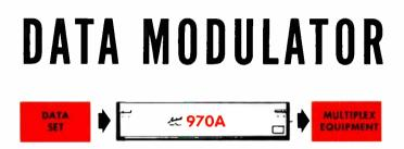
**Lenkurt's 970A Wideband Modulator** converts the output frequency of high-speed data transmission equipment to the group frequency range of carrier and radio multiplex. The set works with 12, 24, and 40.8 kb/s data modems, and includes equalizer sections to compensate for envelope and delay distortion on cable routes. For details, write Lenkurt, Dept. B720.
