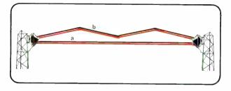
Figure 6. With frequency diversity two wavelengths travel the same refracted path (b) but will not have the same interfering effect on the direct wave (a).
