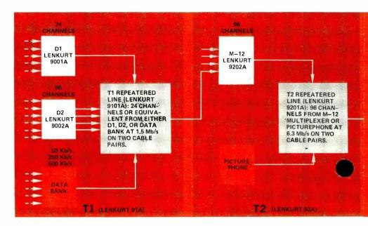
Figure 2. PCM systems, expanding from T1 to T4, will mix voice and other
