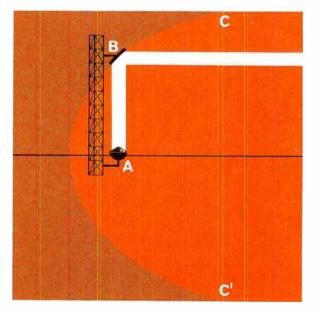
Figure 5. To calculate the curve of a periscope reflector (B), it is convenient to consider the illuminating dish (A) as the focal point of the parabola represented by  $CC^1$ . The reflector (B) may simply be considered a solid segment of the imaginary parabolic shell.
