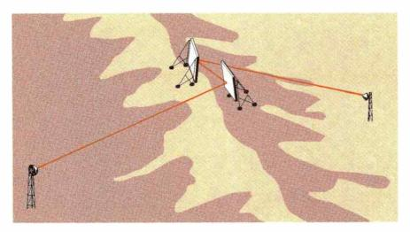
Figure 7. Double passive used to beam signal over a ridge.
