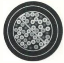
Figure 3. T-Screen cable uses an insulated shield to separate conductors effectively into two channels, thus reducing far-end crosstalk (FEXT), particularly for PCM transmission.
