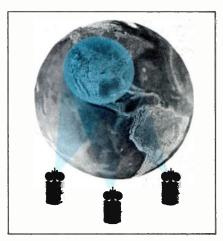
Figure 1. A domestic satellite system would use a series of synchronous, geostationary satellites for communication with all parts of a country.
