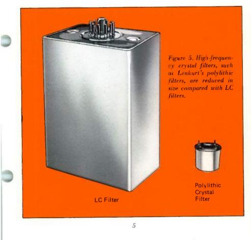
In designing a crystal filter for a particular resonant frequency, the desired information from the computer is the crystal size and shape and the dimensions of the electrodes. For multi-electrode crystal resonators, the spacing of the electrodes is also necessary. Using established computer programs, it is possible to calculate the component values for an equivalent LC resonator and from these values, the crystal filter requirements.
