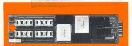
LENKURT'S 5540A FOUR-WIRE TERMINATING UNIT has eliminated the traditional use of separate pads or strappable terminals for attenuation adjustments between four wire facilities and two-wire office equipment. Other advantages of the 5540A include improved performance, low cost, compact size, and front-access test points. For more information, write Lenkurt, Department C134.
