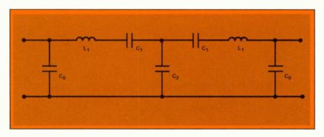
Figure 6. By knowing the values of the four electrical components illustrated, the equivalent two resonator crystal can be designed.
