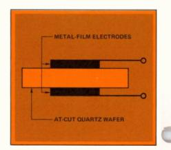
Figure 1. High-frequency crystal resonators have metal-film electrodes plated on the surface of AT-cut quartz crystal wafers.
