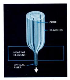
Figure 2. Fiber optics can be made from a glass rod placed inside a glass cylinder of a lower index of refraction.
