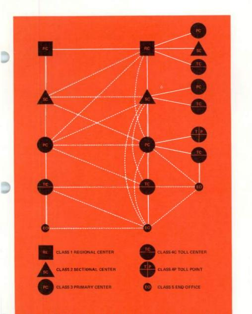
Figure 1. Hierarchical structure of the telephone switching network in the United States. Solid lines indicate main lines of connection within the hierarchy; dashed lines show examples of so-called "high-usage tranks" that can be connected between any two offices (regardless of rank) whenever the traffic volume justifies it.
