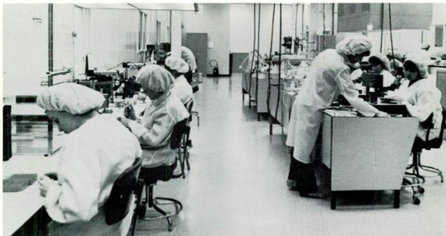
Figure 3. Integrated circuits, hybrid film circuits, and polyolithic crystal filters are constructed in a clean-room environment.
