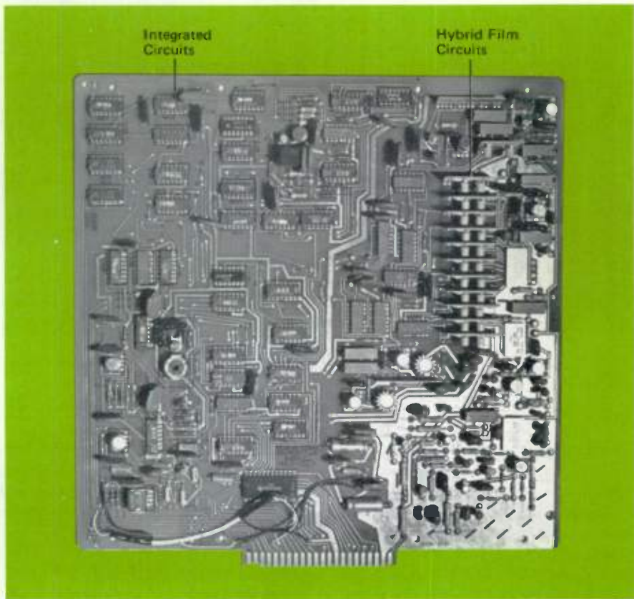
Figure 1. Modern telecommunications equipment subassemblies widely employ the use of integrated and hybrid film circuits.
