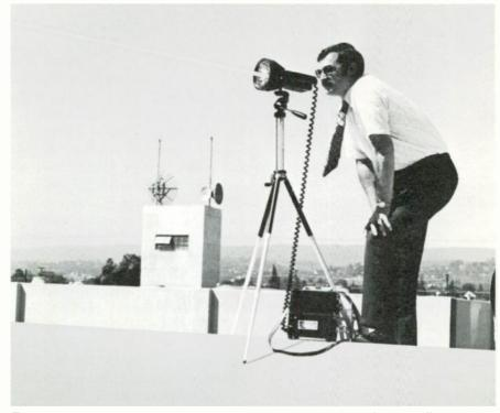
Figure 4. A searchlight provides an efficient method of "flashing" a path in daylight and poor visability at distances up to 30 miles.
