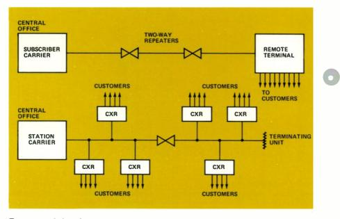
Figure 2. Subscriber carrier systems distribute customer lines from locally powered remote terminals. Station carrier terminals are powered from the central office and are randomly distributed along the line.
