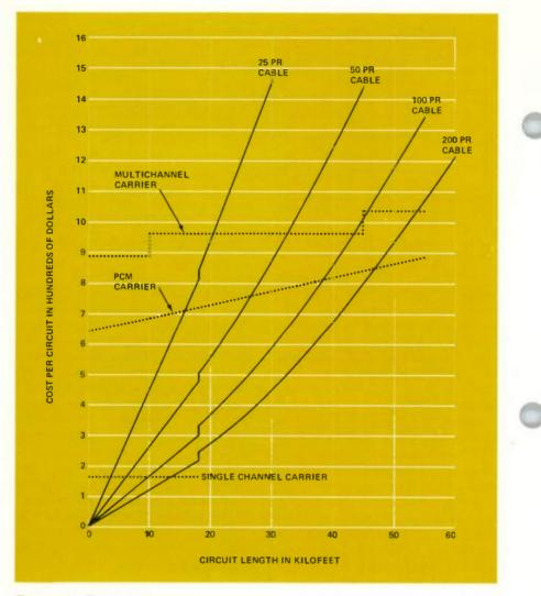
Figure 4. Typical example of comparison of in-place costs for single and multichannel subscriber carrier versus buried cable, with a  $1200\Omega$  customer loop-resistance limit. Beyond the crossover point, the in-place cost of carrier is more economical than cable plant.
