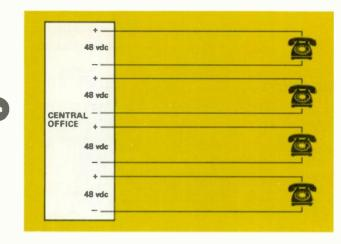
Figure 1. Prior to carrier, each subscriber line was powered by the central office and required one physical cable pair per customer circuit.
