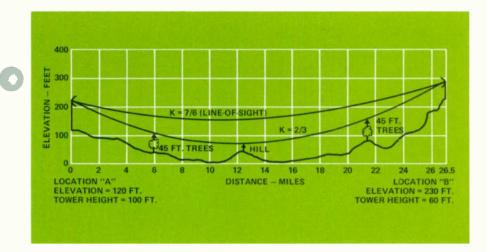
Figure 1. A tentative path profile can indicate the critical points that should be checked in the field.
