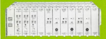
The 54A provides wideband communications services utilizing frequencies above the normal baseband on microwave radio transmission facilities. It is suited for transmitting the audio portion of a TV program, for wideband data, and for multiplex applications. For more information write GTE Lenkurt, Department C134.
