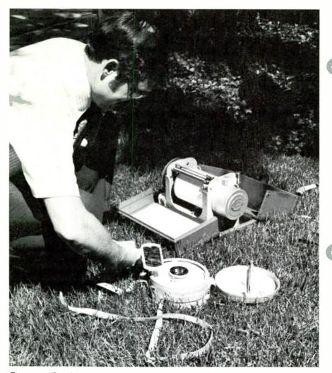
Figure 2. The barograph and the roving altimeter are calibrated to a known elevation at the beginning of the survey and rechecked at the conclusion.
