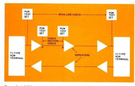
Figure 5. A PCM test set can be used to check cable pairs between repeaters, and entire repeatered lines.
