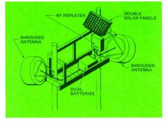
Figure 5. An rf repeater pole installation.
