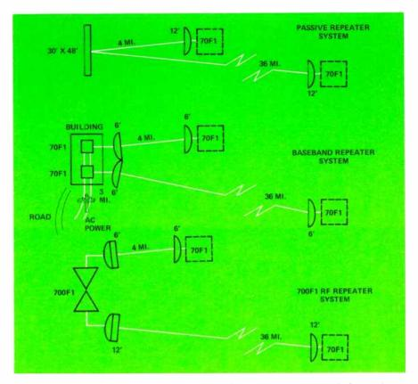
Figure 3. The use of an rf repeater can provide a simple, economical alternative to narrowband repeater applications.
