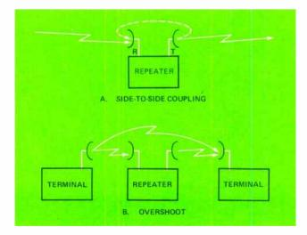
Figure 2. Side-toside coupling and signal overshoot are two types of interference that may exist at a repeater location.
