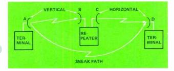
Figure 7. Cross-polarization of antennas can reduce the effects of delay distortion caused by "sneak" paths.
