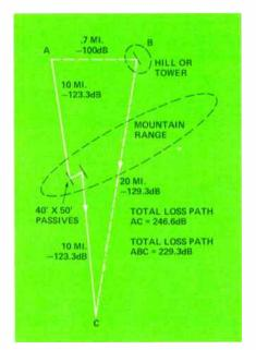
Figure 6. An rf repeater offers improved gain and economy in straightline path narrowband applications.
