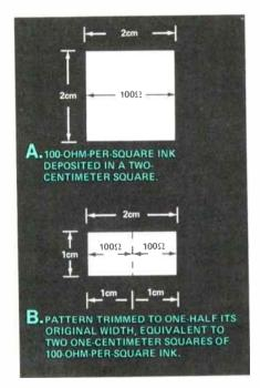
Figure 4. The relationship of length to width in thick film resistors is linear, allowing values to be easily changed by trimming techniques.
