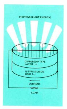
Figure 2. Operation of a typical silicon photodiode. Such cells can be arranged in series/parallel circuits to obtain the desired output.
