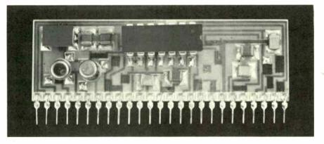
Figure 1. Thick film hybrids combine discrete-component and monolithic technologies to produce circuits that retain many of the advantages of both.
