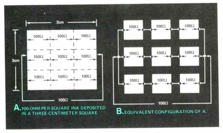
Figure 3. The resistance of a thick film resistor is a function of shape rather than size.
