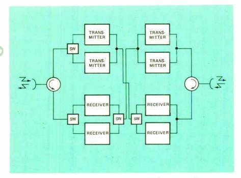
Figure 4. A typical microwave repeater facility including hot-standby protection. Such repeater sites require power for every active element, as well as backup batteries to provide service during power outages.
