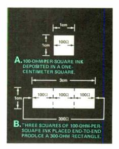
Figure 2. Thick film resistors are formed with special inks whose values are specified in "ohms per square."
