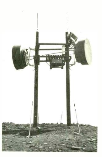
Expensive honsing is unnecessary for the 700F1, which operates over a temperature range of  $-40^{\circ}$ F to  $+140^{\circ}$ F and has all its active components mounted in a weatherproof metal box. Since the 700F1 uses a minimum of components, it is more reliable than conventional repeaters; in addition, the entire system is 100 percent actively redundant.
