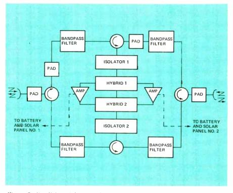
Figure 5. Simplicity of design and the elimination of the frequency conversion process permits the GTE Lenkurt 700F1 RF Repeater to operate on less than four watts of power. Storage batteries provide 10-day backup capability for periods of prolonged darkness.
