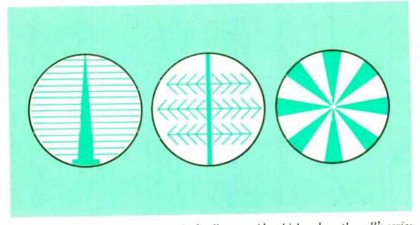
Figure 1. These patterns are typical of collector grids which reduce the cell's series resistance. Square and rectangular cells usually have grids in finger-shaped patterns.
